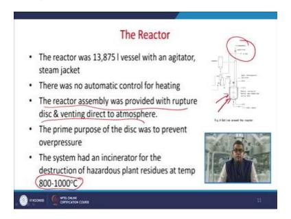
Now let us have a brief look about the reactor. The reactor was 13875 liter of vessel with an agitator and steam jacket and there was no automatic control for heating. The reactor assembly
