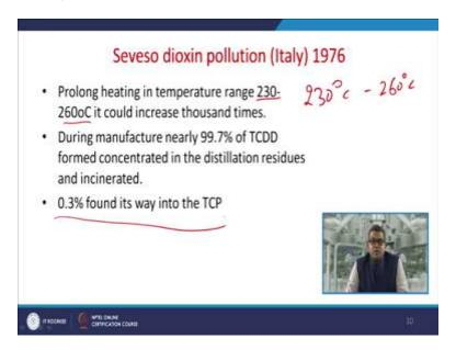
Now if you go on the prolong heating in the temperature range of 230 to 260 degrees Celsius, it could increase the thousand times. So, during the manufacturing or during the process nearly 99.7 percent of TCDD formed concentrated in the distillation residues and incinerated. Now only (1) 0.3 percent, 0.3 percent found its way into TCP.
