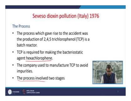
Now let us have a discussion about the process, the process which gave rise to the accident was the production of 2, 4, 5 trichlorophenol TCP is in a batch reactor. Now, this trichlorophenol is required to for making the bacteriostatic agent called hexachlorophene. Now the company used to manufacture this trichlorophenol to avoid any kind of impurities. Now this process involved two stages.
