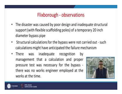
So this disaster was caused by poor design and inadequate structural support with the (flexible) jack-knife type of scaffolding of a (temperature) temporary 20-inch diameter bypass pipe. Now the structural calculation for the bypass were not carried out, such calculations might have anticipated the failure of mechanism. So again, they have, you can say they have missed this particular aspect, a very important aspect of the process.
