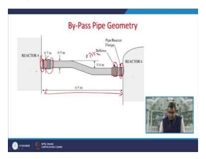
Now this was the bypass pipe geometry, this was a reactor 4 and this was a reactor 6, they were supported by these bellows and the pipe reactor flanges and the distance was almost 355 meter just to suggest that reaction kinetics and the distance of these two reactors, remember reactor 4 to reactor 6 was 6.5 meter.
