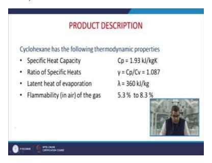
Now cyclohexane is having the following thermodynamic properties like specific heat is 1.93 kilo joule per kilogram kelvin, ratio of specific heat that is gamma is equal to 1.087, latent heat of evaporation is 360 kilo joule per kilogram and flammability in air of the gas is 5.3 to 8.3, in other words you can say the LFL and UFL.
