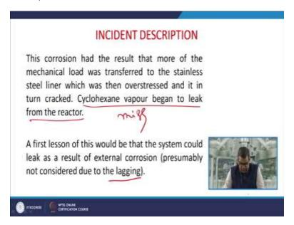
So this correction had to the had the result that more of the mechanical load was transferred to the stainless steel liner which was then overstressed and it in turns cracked. So cyclohexane vapors they begin to leak from the reactor, again you can say this is the miss. Now the first lesson of this would be that the system could leak as a result of an external corrosion that is presumably not considered to due to the lagging. So sometimes it may referred as that this is lagging but it is not.
