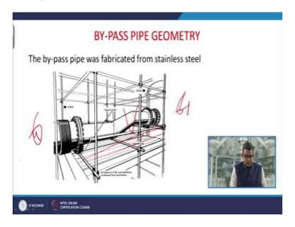
Now this was the structure of scaffold and this you can see the scaffold which was supported the reactor number 4 to reactor number 6.
