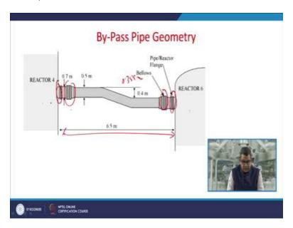
Now you can see in this particular figure that whenever the flow is transferred from this way. So the load would be on the higher side of this particular pipe junction.
