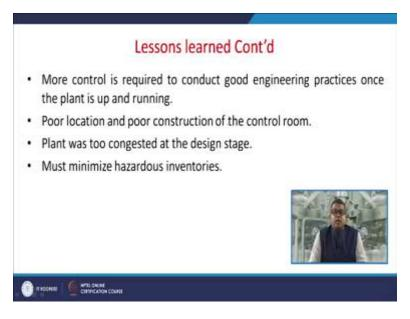
The more control is required to conduct a good engineering practices once the plant is up and running, that means the top at that particular point of time the workers, they were not well trained because they carry out all kind of bypass analysis through chalk on the maintenance floor. The poor location and a poor construction of the control room because it was collapsed at the time of vapor cloud explosion. The plant was too congested in that design (state) stage.
