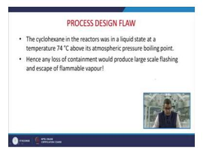
Now there are certain process design flaw, the cyclohexane in the reactor was in a liquid state at a temperature of 74 degrees Celsius above its atmospheric pressure boiling point. Hence any loss of containment would produce large scale of flashing and escape of flammable vapor. Now the cyclohexane and the benzene both of them they were stored in a large quantity, so inventory problem was also there in that particular thing.
