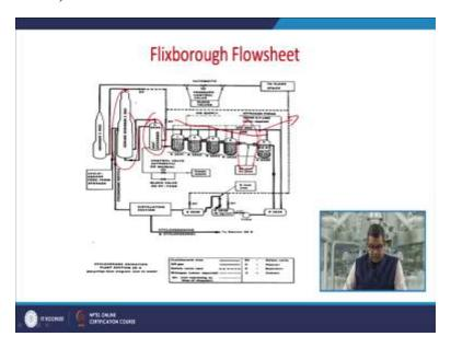
So if you recall, the production protocol, so these 6 reactors they were in series and the overflow of the previous reactor is subjected to the inlet of the next reactor inline and in such a way. So
