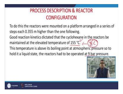
Now since to meet the reaction kinetics, they were having the 6 reactor in series. Now to do this the reactors they were mounted on a platform arranged in a series step such that each step is having the height difference of 0.355 meter with another one. Now, the good reaction kinetics, they dictate that the cyclohexane in the reactor be maintained at an elevated temperature of 155 degrees Celsius.
