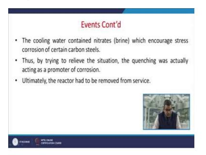
And this cooling water contained nitrates, brine just to have a thermodynamic calculation. So which (can) encourages the stress corrosion of certain carbon steel. So thus by trying to relieve
