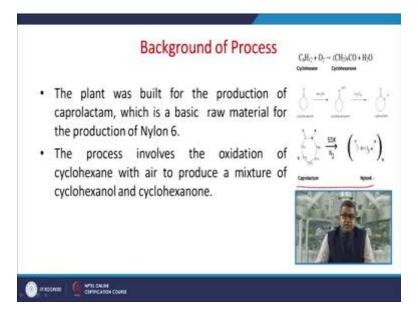
Now let us have brief discussion about the process. The plant was built for the production of caprolactam which is basic raw material for the production of nylon-6. Now the process involves the oxidation of cyclohexane with air to produce a mixture of cyclohexanol and cyclohexanone
