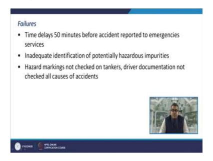
There was a time delay of 50 minutes before accident reported to emergency services. There was an inadequate identification of potentially hazardous impurities and hazard marking was also not checked on the tanks, driver documentation not checked, all the causes of accident. The reason was that because the source of ignition was unknown and it practically investigation team failed to find out the source of ignition from which that vapor cloud was ignited.
