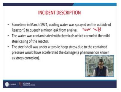
So sometimes in March 1974, the cooling water was sprayed on the outside of reactor number 5 to quench a minor leak from a valve. Now the water was contaminated with the chemicals which corroded the mild steel casing of the reactor. Now this problem you can say, this is the near miss. Now the steel shell was under a tensile hoop stress and due to this the contained pressure which would have accelerated the damage. Now this phenomenon is known as the stress corrosion.
