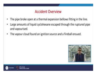
Now the pipe broken down, open at a thermal expansion bellow fitting in the line, the large amount of liquid cyclohexane escape to the atmosphere through the rupture pipe and vaporized because they were having the higher temperature and excess pressure. So the vapor cloud found an ignition source and a fireball in ensued.
