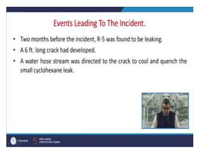
Now 2 months before the accident, the reactor number 5 was decommissioned and because they were founded to be leaking, a 6 feet long crack there in that particular reactor was developed, a water hose stream was directed to crack, to the crack to cool and quench the small cyclohexane leak.
