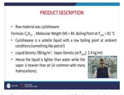
Now let us a Product Description, so the raw material for that particular caprolactam production was cyclohexane, it is having the formula of C6 H12 molecular weight 84 and boiling point is 81 degree Celsius. Now this cyclohexane is a volatile liquid with a low boiling point at ambient condition. It is something like petrol. It is having the liquid density, 780 kilogram per meter cube
