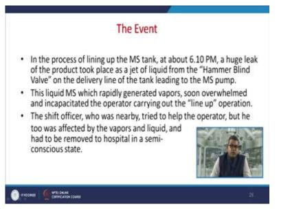
So in the process of lining up MS tank at around 6:10 p.m. a huge leak of the product took place as a jet of liquid from the hammer blind valve on the delivery line of the tank leading to the MS pump that is motor spirit pump. Now this liquid petrol which rapidly generated a vapours and soon overwhelmed and incapacitated the operators carrying out the line of operation.
