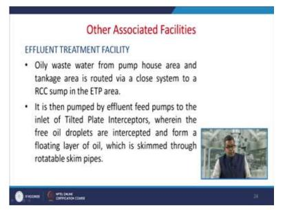
Apart from other things they were having the effluent treatment facilities so oily waste water from the pump house area and tankage area is routed via a closed system to a RCC sump in the effluent treatment plant. Now, it is usually then pump with a effluent feed pumps to the inlet of tilted plate interceptors where in the free of oil droplets they are intercepted and form a floating layer of oil, which is skimmed through a rotatable skim pipes.
