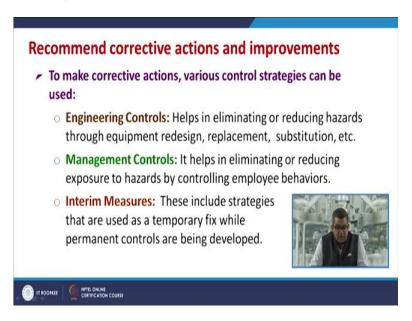
Now to make the corrective action various control strategies can be used, one is the engineering control this helps in eliminating or reducing hazard through equipment redesign and replacement, substitution, attenuation, isolation etc. Then the Management control it helps in eliminating or reducing exposure to hazard by controlling employee behaviour the third one is the interim measures. These include the strategies that are used as a temporary fix while permanent controls are being developed.
