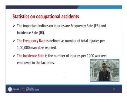
Now, the important indices on injuries are frequency rate that is FR and incidence rate that is IR now the frequency rate is defined as number of Total injuries per 100000 man-days worked. This one and the incidence rate is the number of injuries per 1000 worker employed in those factories or establishments.
