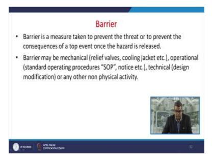
Now let us have a look about the barriers so the barriers they are the measures taken to prevent the threats or to prevent the consequences of a top event once the hazard is released. So this barriers may be mechanical like relief valve, cooling jackets etc. operational like standard operating procedures SOPs, notices etc. there may be technical that is the design modification or any other non-physical activity.
