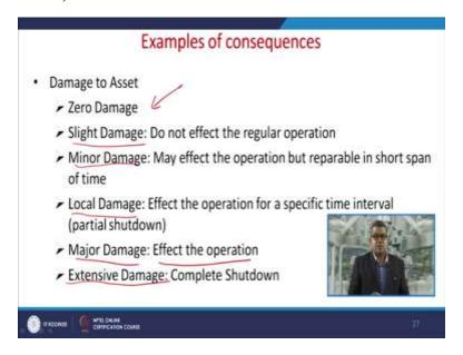
Other examples of like that damage to asset sometimes it may happen that there is no damage at all in the plant then there may be a consequence of slight damaged they do not effect the regular operation so slight effect may take place and then there is no process loss or any kind of hampering towards the regular operation. There may be certain minor damage this may affect the operation but it can be repaired in a short span of time.
