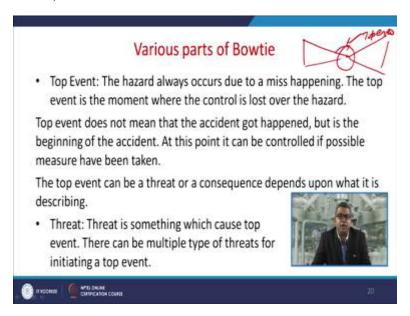
Next aspect of the Bowtie part is the top event the hazard always occurs due to the miss happening the top event is the moment where the control is lost over that particular hazards. So you are not having any kind of things which you need to control. Top event does not mean that the accident got happened but is the beginning of the accident.
