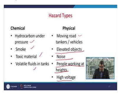
Now there are various type of hazards like chemical hazards and the physical hazards couple of examples are chemical hazards that are hydrocarbon under pressure, smoke, toxic materials, volatile fluids in tanks there may be certain physical hazards like moving road tankers or vehicles, elevated objects, noise, people working at height and sometimes the high voltage.
