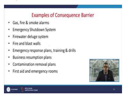
The other example of consequence barriers like gas, fire and smoke alarms, emergency shutdown system. You may have a firewater deluge system, the fire and blast walls, the emergency response plans training and drills, you may have a business resumption plan, contamination removal plans also clubbed under the head of consequence barrier. The first aid and emergency rooms.
