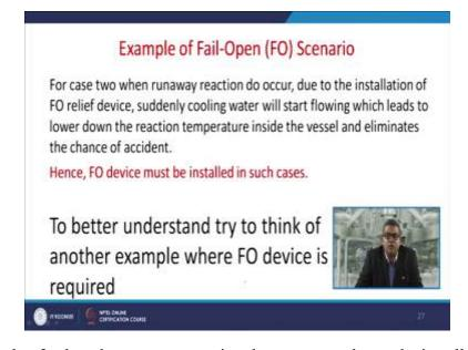
For the case number 2 when the runaway reaction do occur now due to the installation of this fail-open relief device suddenly cooling water will start flowing which leads to lower down the reaction temperature inside the vessel and eliminates the chance of accident hence the fail-open device must be installed in such a cases. So to better understand try to think of another example where fail-open device is required.
