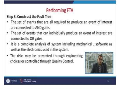
Now the next step is the construction of fault tree, the set of events that all required to produce and event of interest are connected to an AND gate then the set of events that can individually produce an event of interest are connected to OR gate, it is a complete analysis of system including mechanical, software as well as the electronics used in the system. Now this risk may be prevented through engineering choices or control through quality control.
