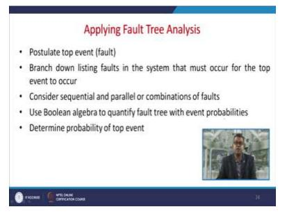
Now while considering the (applic) applying the fault tree analysis you must postulate the top event that is the fault then branch down the listing fault in the system that must occur for the top event to occur, must consider the sequential and parallel or combination of the fault, use Boolean algebra to quantify the fault tree with event probabilities you need to determine the probability of the top event that is once you have postulated the top event that is fault.
