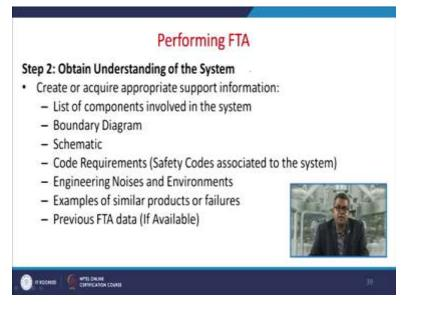
Now the second step is to obtain the understanding of the system, this create or acquire the appropriate support in formation, this includes the list of the components involved in the system, boundary diagrams, schematic diagrams, code requirements, that is safety code associated to the system, engineering noises and environments, example of similar product or failures and in case if you have any previous fault tree analysis data it should be included.
