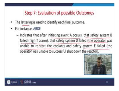
Now the next step is the evaluation of a possible outcome so the lettering is used to identify the each final outcome, for instance ABDE in this the indicates that after initiating event A occurs the safety system B failed that is high temperature alarm the safety system B failed the operator
