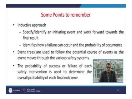
Now there is one approach called inductive approach in this approach you need to specify or identify an initiating event and work forward towards the final result. This identifies how a failure can occur and what is the probability of the occurrence of that particular failure?
