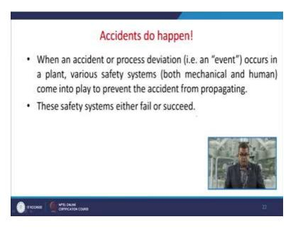
Now accidents they do happen so when accident or process deviation that is an event occurs in a plant various safety system both mechanical and human come into play to prevent the accident from propagation. Now these safety system either fail or succeed.
