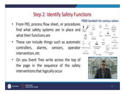
Then you identify the safety functions so from PID process flow sheet or a procedure find what is safety systems are in place and what their functions are? So here we have enlisted different P&ID symbols for various valves like Bleeder valve, Gate valve, Ball etc. Now this can include things such as automatic controllers, alarms, sensors, operator interventions etc. So on you Event tree write across the top of the page in the sequence of safety interventions that logically occurs.
