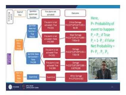
The horizontal lines they are drawn between the function that applies here you have applied the horizontal lines. Vertical lines are drawn with each safety functions that applies like success upward, failure downward and no effect there would be no branch at all. Now indicate the result of event that is circle you may indicate with the acceptable result, the cross circle that is unacceptable result like this.
