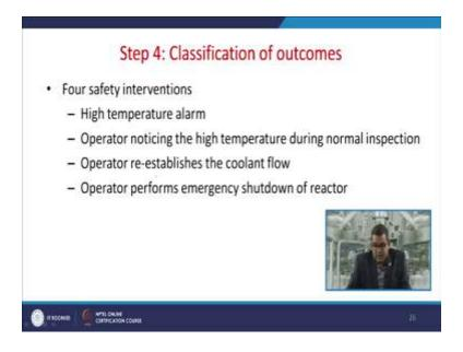
Our next step is that you need to classify the outcomes, now there are four safety interventions one is that high temperature alarm, sometimes the operator notice in the high temperature during the normal inspection when operator reestablishes the coolant flow sometimes because of the failure of this things so he actually reestablish the cooling flow and then operator performs the emergency shutdown of reactor.
