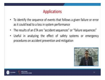
Now let us talk about the applications of this ETA, to identify the sequence of event that follows a given failure or error as it could lead to a loss in system performance the result of an event tree analysis are accident sequences or failure sequences they are useful in analyzing the effect of safety system or emergency protocols or procedure on accident prevention and mitigation.
