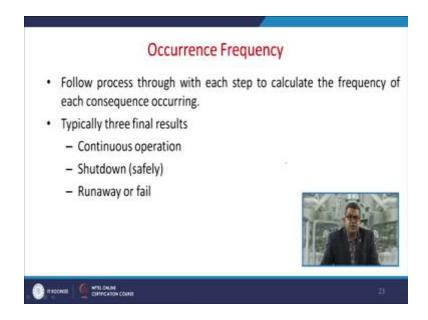
So we must look into the occurrence frequency so the follow the process through which each step to calculate the frequency of each consequence occurring now typically there are three final results maybe in terms of continuous operation, may be the safe shut down or may be the run away or a failure. So you have to look into three different results.
