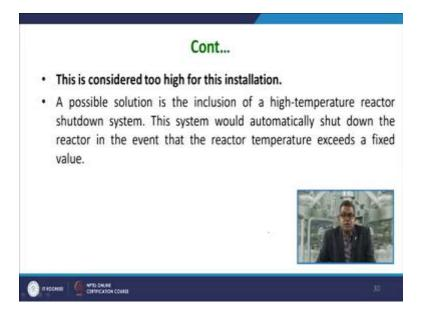
So this is considered too high for this type of installation. Now possible solution of this inclusion of high temperature reactor shutdown system this system would automatically shutdown the reactor in the event that the reactor temperature exceeds a fixed value.
