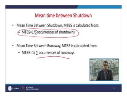
Now there is a concept of Mean Time between the shutdown so you need to evaluate this one the mean time between the shutdown MTBS is calculated from this formula MTBS is equal to 1 upon summation occurrence of all kind of shutdowns. So the Mean Time Between the Runaway reactions MTBR is calculated by this one MTBR is equal to 1 upon summation of occurrence of various Runaways.
