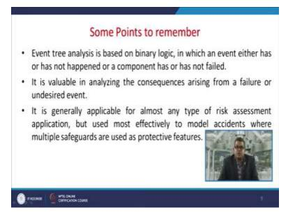
So there are certain points you need to remember and those points are that event tree analysis is based on binary logic in which an event either has or has not happened or compared has or has not failed. So there are only two option either this work or will not work. So it is a valuable in analyzing the consequences arising from a failure or undesired event. It is generally applicable
