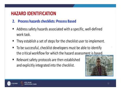
Now, there are 2 basic type of checklist one is that process based another one is the behaviour based. Now, let us have a look about the process based checklist, this addresses the safety hazard associated with a specific well defined work task. Now usually they establish a set of
