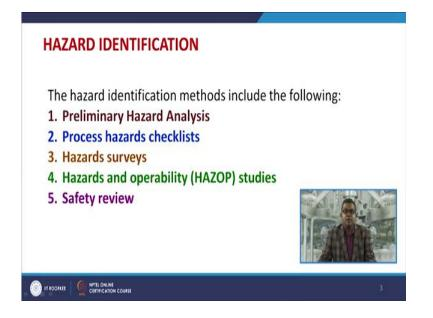
So, in continuation to that particular aspect the hazard identification methods this may include the following aspect like preliminary hazard analysis, then we have to construct the process hazard check list on the basis of the different hazard analysis and identification protocol. Then we need to perform the hazards surveys, go for the hazard and operability studies that is called the HAZOP studies and we need to perform the safety reviews.
