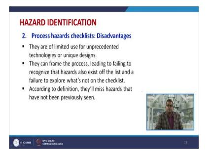
Then we are having so many advantages of these process hazard checklist there are certain disadvantages. Now, these disadvantages are they are limited use of unprecedented technologies or unique design. They can frame the process leading to, failing to recognize the hazard also exist in the list and a failure to explore what is not on the checklist, sometimes you may overlook any kind of things which need to be listed in checklist.
