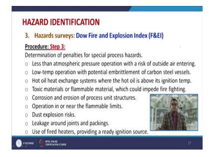
The next step is the determination of a penalties for special process hazards that is less than atmospheric pressure operation with risk of outside air entering, so that there may be a chance of flammability. Low temperature operation with the potential embrittlement of carbon steel vessel. Hot oil heat exchange system where the hot oil is above its ignition temperatures sometimes it may lead to the auto ignition scenario.
