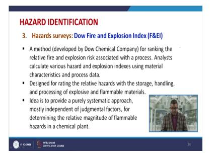
So let us have a look of the one by one, the first one is the Dow fire and explosion index, F&EI that is a method developed by the Dow chemical company for ranking the relative fire and explosion risk associated with the process. Now, analysis, the analyst calculate the various hazard and explosion indexes using the material characteristics and process data available.
