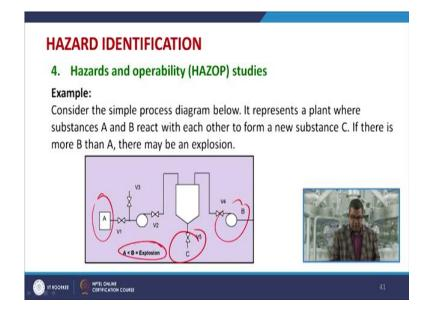
Now, one example is that consider a simple process diagram this figure it represents a plant where a substance A and B reacts with each other to form a new substance that is called C. There is if there is more B then A there may be an explosive, so this is the chance of explosive. (Refer Slide Time: 31:55)
