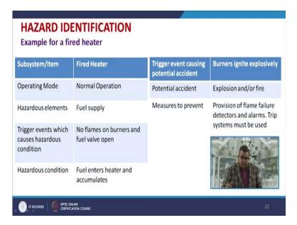
Now, let us have an example of a fired heater. This gives you a good clue about this PHA. There are various subsystems and item like operating mode sometimes fired heater normal operation hazardous element may present like that is called the fuel supply. The triggered event which is which causes the hazardous condition that may be no flame on the burners or a fuel valve open.
