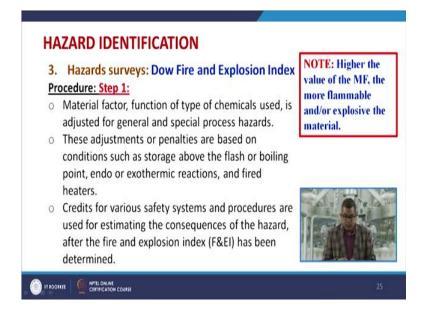
Now, this is a multistep process and the first step in this to perform the hazard survey pertaining to the Dow fire and the explosion indexes the material factor, function of type of material used, is adjusted for the general and special process hazard. Now, these adjustment or penalties are based on the conditions such as storage above the flash or a boiling point, endo or exothermic reactions and fired heaters.
