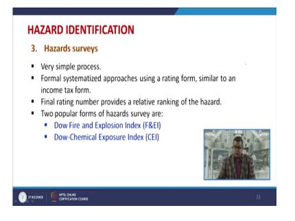
Now, these hazards surveys are very simple process as we have shown in the, this particular slide. These are the simple questions which you need to ask, then formal systematized approach using a rating form similar to an income tax form. Now final rating number provides a relative ranking to the hazard. Now, there are 2 popular forms of hazard surveys they are, one is the Dow Fire and Explosion Index that is F&EI another one is the Dow Chemical Exposure Index that is CEI.
