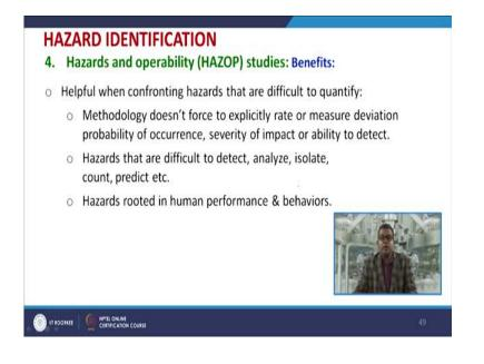
The methodologies does not force to explicitly rate or measured deviation probability of occurrence severity of impact or ability to detect. The hazards that are difficult to detect, analyse, isolate, count, predict etc. These hazards are rooted in human performance and behaviour.
