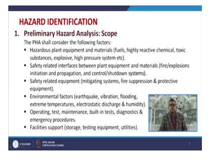
Let, us have a look about the scope of the preliminary hazard analysis. This shall consider the different factors like hazardous plant equipment and materials like fuel, highly reactive chemical, toxic substances, explosives, high pressure systems, etc. Then the safety related interfaces between the plant equipment and material again the examples are the fire explosion initiation, propagation and control shut down systems.
