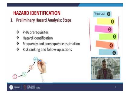
Now, there are various steps involved in this preliminary hazard analysis one is so we are going to in detail, that what has the PHA prerequisites. You must have a proper hazard identification list with you, you must have a frequency and a consequences estimation, then you must have a risk ranking and a follow up action. So by this way you can go for this to do list.
