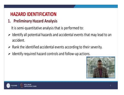
So, let us have a look about the first task right that is the preliminary hazard analysis this is some sort of a semi quantitative analysis that is performed to identify all potential hazards and accidental events that may lead to an accident. So, you need to identify all those things, then basis of your, on the basis of your identification you need to 1rank the identify the accidental event according to their severity. And then identify the required hazard control and follow up actions.
