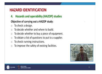
Now, there are set of objectives carrying out for the HAZOP study. One is to check the design whether it is proper or improper. To decide whether and where to build the things to decide whether to buy a piece of equipment or not, to obtain a list of a questions to put to a supplier, to check running instruction that may be imposed to a worker, to improve the safety of any existing facilities.
