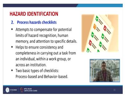
Now, next step is that the process hazard checklist now this is attempt to compensate for the potential limit of hazard recognition, human memory and attention to specific details. This helps to ensure the consistency and completeness in carrying out a task from an individual within a workgroup or across an institution.
