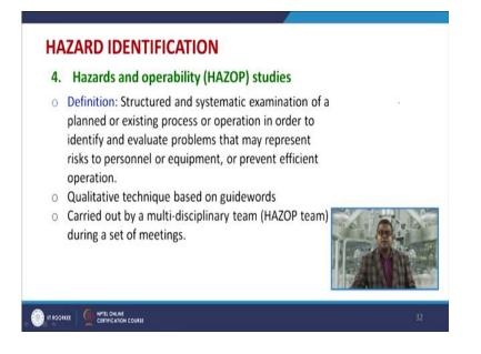
Now, next is the Hazard and Operability Studies (HAZOP). The basic definition of this HAZOP is that this is structured and systematic examination of plant or existing process or operation, in order to identify and evaluate problem. That may represent risk to personal or equipment or prevent efficient operation. This is the qualitative technique based guidewords carried out by multidisciplinary team that is called the HAZOP team during the set of meeting.
