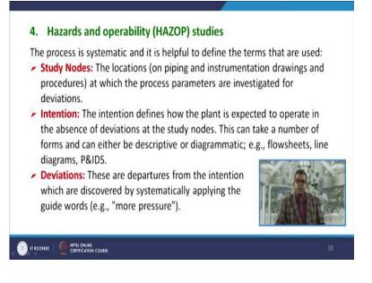
Now, this process is systematic and it is helpful to define the terms that are used like study notes the location for example on piping and instrumentation drawing and procedure. The location at which the process parameters are investigated for deviation. Then the intention, the intention defines that how the plant is expected to operate in absence of deviation at the study nodes.
