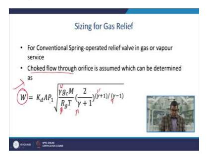
Then we can go for the sizing of for Gas Relief. So this is for the conventional spring-operated relief valve in gas or a vapor service. So choked flow through orifice is assumed which can be determined by this equation. Remember we have already discussed this choked flow in the previous modules. Now, this is defined as
