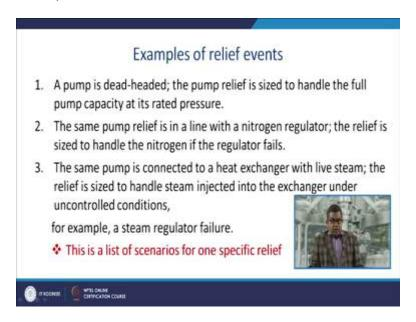
Now, let us have a couple of example for the relief event. Now, a pump is dead-headed, the pump relief size to handle the full pump capacity at its rated pressure. Now the same pump relief is in
