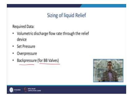
So, whenever we perform the sizing of liquid relief, we are required various set of data that the volumetric discharged flow rate through the relief device that depends on the opening of the relief device. What is the set pressure of that relief device? What is the due consideration of the overpressure in question or were pressure in the process? And we need to consider back pressure especially for BB valves.
