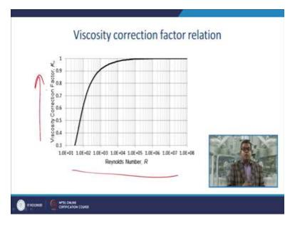
Now, another is the viscosity correction factor relationship here this particular standard curve is with respect to the Reynolds number and viscosity correction factor Kv, so here in the X-axis we
