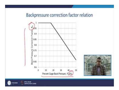
Now this plot shows the back pressure correction factor relation. Now here in the X-axis we are having the back pressure correction factor that is Kw and here the percentage gage back pressure that is Pg in percentage. So you can calculate and you can have a look while you require the back pressure correction factor over this particular equation.
