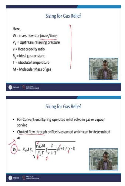
Now, here W, this W is the mass flow rate having the unit of mass per time. P1, this P1 is the upstream relieving pressure, gamma is the heat capacity ratio,  $R_g$  is the ideal gas constant, T is the absolute temperature and M is the molecular mass of gas. So these are the standard denotations of this particular formula.
