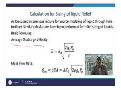
So while performing the calculation for sizing of liquid relief, we have already discussed in the previous lecture of various source model of liquid through different openings or holes or orifice. The similar calculations have been performed for relief sizing of liquid. So the basic formula is almost same. Now, here we have the average discharge velocity that is
