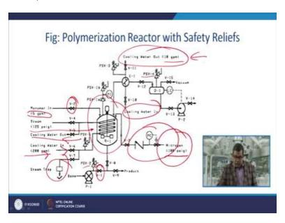
Another is the polymerization reactor with a safety relief. Now, here you are having a polymerization reactor with monomer, the quantity is given that how much the flowrate, this is a valve. Now steam injection, the cooling water out, the cooling water in, so you are having 1, 2, 3, 4 different media, there is an steam trap. Here the nitrogen purging is given to it and this particular reactor is operating under vacuum.
