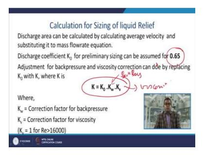
So the discharge area you can calculate by calculating the average velocity. It is a normal fluid dynamics phenomena, the average velocity and substituting it to the mass flow rate equation. Now this K naught is the discharge coefficient for the preliminary sizing, this can be assumed to be at 0.65. So adjustment for the back pressure and velocity correction can be done by replacing  $K_0$  with K, where
