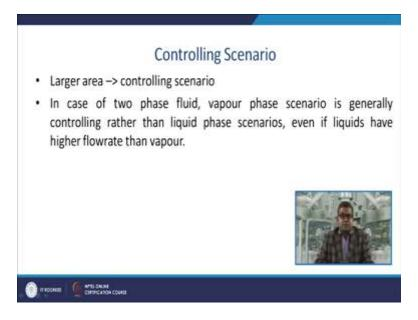
Then we have to discuss about the controlling scenario. Remember, whenever we are having the larger area then the controlling scenario come into the picture. So in case of two phase (flow) fluid vapor phase scenario is generally controlling rather than liquid phase scenario, even if liquid have higher flow rate than the vapor one.
