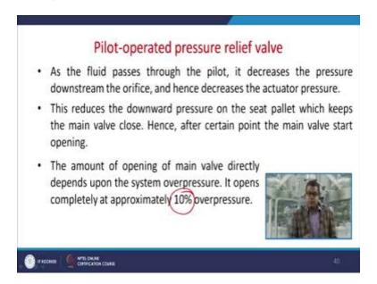
Now as the fluid passes through the pilot, it decreases the pressure downstream to the orifice hence decreases the actuator pressure. Now this reduces the downward pressure on the seat pallet which keeps the main valve closed. So hence after certain pilot, at certain point the main valve start opening. So the amount of opening of main valve directly depends on the system over pressure and it opens completely at the (approx) or you can say, the approximately 10 percent of over pressure.
