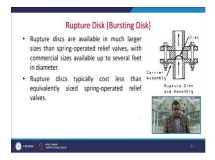
Now these rupture discs are available in much larger size than the spring operated relief valve with commercial sizes available up to several feet in diameter. These ruptured typically cost less than the equivalently sized spring-operated relief valve and moreover the maintenance and other things are on the lower side for these rupture discs compared to the spring operated relief valve where you need to perform the regular maintenance.
