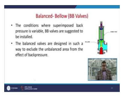
Now the conditions where the superimposed back pressure is variable these balanced bellow valves are suggested to be installed. So the balanced valves are designed in such a way to exclude the unbalanced area from the effect of back pressure.
