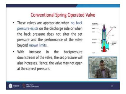
So these valves are appropriate when no back pressure exist on the discharge side or when the back pressure does not alter the set pressure and the performance of the valve known as beyond limit. Now with increase in the back pressure downstream of the valve, the set pressure will also increase hence the valve may not open at a correct pressure.
