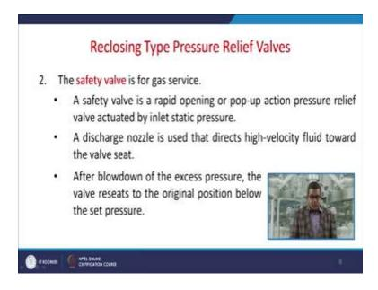
Now if we discuss about the safety valve for the gas service, a safety valve is a rapid opening or pop-up action pressure relief valve actuated by inlet static pressure. A discharge nozzle is sometimes used to direct the high-velocity fluid towards the valve seat. Now after the blowdown of the excess pressure the wall reseats to the original position below the set pressure.
