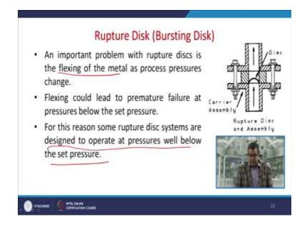
Now an important problem with the rupture disc is the flexing of metal as process pressure changes. So if the process pressure fluctuating then there may be a problem of flexing of the metal. So flexing could lead to the premature failure if the pressures below the set pressure. So this is you may term as the disadvantage. For this reason some rupture disc systems are designed to operate at pressure well below the set pressure. So this is the crucial aspect.
