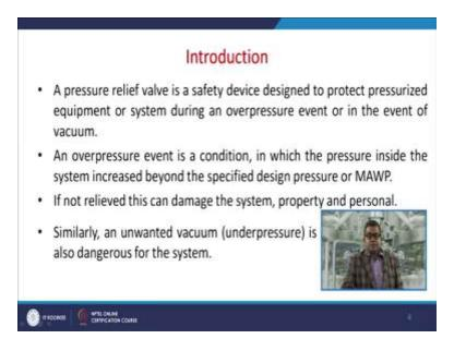
Now a pressure relief valve is safely designed to protect the pressurized equipment or system during an overpressure event or in the event of vacuum. Now an overpressure event is a condition in which the pressure inside the system increased beyond the specified design pressure or MAWP, Maximum Allowable Working Pressure. Now if not relieved this can damage the
