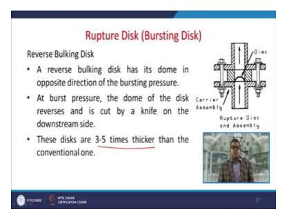
Now we have a reverse bulking disc. Now a reverse bulking disc has its dome in opposite direction of the bursting pressure. At burst pressure the dome of the disc reverses and it cut by a knife on the downstream side. Now these discs are 3-4 times thicker than the conventional one which we have discussed earlier.
