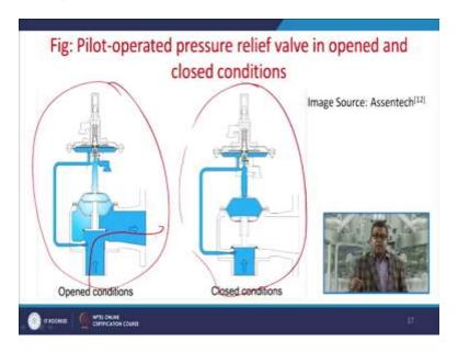
Now this is the typical figure of pilot-operated pressure relief valve in open and closed system. Now this is the open condition, so when fluid passes through this way and this one is the closed one. So you can see all the things which we have discussed in the previous slide, they are here.
