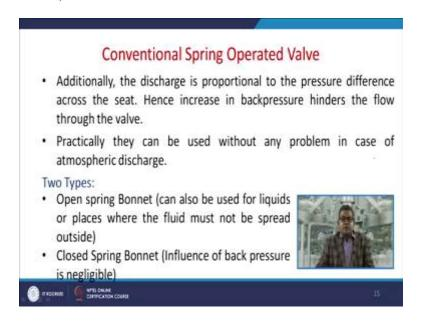
Now additionally, the while discussing the conventional spring-operated valve additionally the discharge is proportional to the pressure difference across the seat. So hence the increase in the
