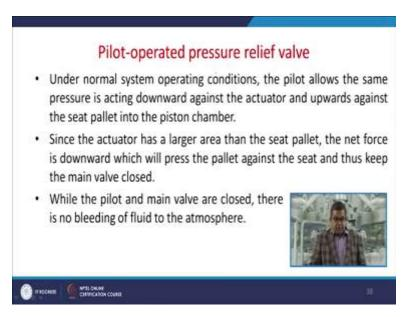
So under normal operating conditions, the pilot allows the same pressure which is acting downward against the actuator or upward against the seat pallet into the piston chamber. Now since the actuator has a large area then the seat pallet, the net force is downward which will press the pallet against the seat and thus keep the main valve closed. So while the pilot and the main valve are closed there is no bleeding of fluid to the atmosphere.
