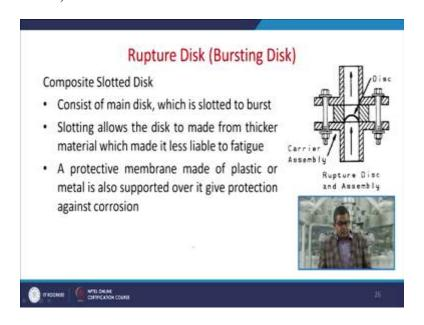
Now let us have a brief discussion about the composite slotted disc, this consists of a main disc (where) which is slotted to burst. Now slotting allows the disc to made from thicker material
