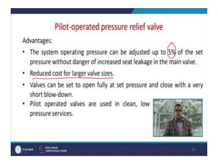
So, there are several advantages associated with this pilot operated pressure relief valve, the system operating pressure can be adjusted up to 5 percent of the set pressure without danger of increased seat leakage to the main valve. They reduced the cost for the larger valve size. Valves can be set to open fully at set pressure and closed with a very short blow down. The pilot operated valves they are used in clean, low pressure services.
