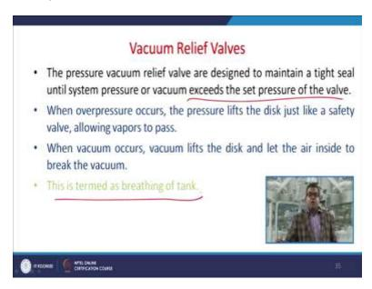
Now the pressure vacuum relief valve they are designed to maintain a tight seals until system pressure or vacuum exceeds the set pressure of the valve. So when the over pressure occurs the pressure lifts the disc just like safety valve allowing the vapors to pass and the when vacuum occurs the vacuum lifts the disc and let the air inside to break the vacuum. Now this is termed as (the) breathing of tank.
