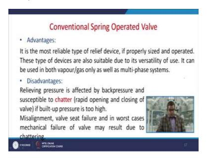
Now there are certain things related to the advantages of these conventional spring operated valve. So it is most reliable type of relief device if properly sized and operated. Now these type of devices are also suitable due to its versatility of use, it can be used in both vapor gas only as well as multi-phase systems. When we are having the advantage, there are certain disadvantages also associated with these conventional spring-operated valves.
