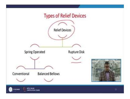
Now here, you can have a look of about the classification stream, these are the relief devices they are further divided into the spring operated one and the rupture disc one. Now spring operated one again they are further classified in two aspect, the conventional and the balanced bellow.
