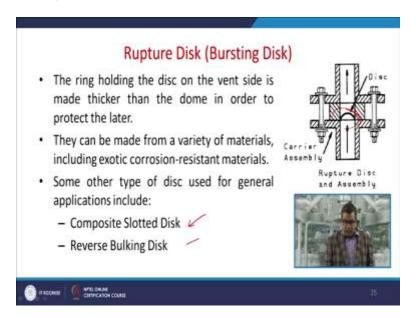
Now the ring holding the disc on the vent side is made thicker than the dome in order to protect it later. Now here, there is a ring. Now this can be made from a variety of the material including exotic corrosion-resistant material etc. Now some other type of disc used for the general application include composite slotted disc, reverse bulking disc.
