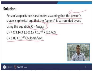
Now while we are considering the solution, the person's capacitance is estimated assuming the person's shape is spherical, that is purely an assumption, remember. And that is the sphere is surrounded by air, so if you use this particular equation which we have studied in the previous module,
