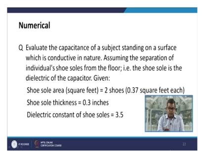
In this particular numerical example, we need to calculate the capacitance of a subject standing on a surface which is conductive in nature. Assuming the separation of individual's shoe soles from the floor, that is the shoe sole is the dielectric capacitor, now you are given the shoe sole area which is in square feet to choose 0.37 square feet each. Shoe sole thickness is 0.3 inches and dielectric constant for shoe sole is 3.5.
