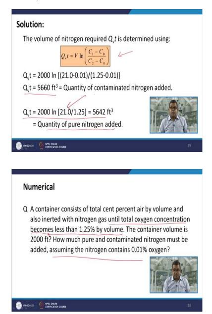
So while we consider the solution, the volume of nitrogen required  $Q_vt$  is determined by using this particular formula  $Q_vt$  which we have already discussed in the previous modules. So,
