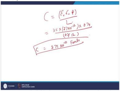
Let us calculate the things. Now individual's capacitance can be estimated assuming the subject shoe sole, and the floor are parallel to each other, so considering the case of 2 parallel plates,
