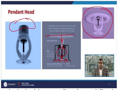
Now this is the pendant head and they are usually roof-mounted. Here the roof is there, so they are roof-mounted. Now here is the anatomy of the pendant head: This is the water supply line and usually the CPVC plastic pipe, nowadays we are using this CPVC plastic pipe. Now here is the bulb. The bulb burst and when it burst then there is a release of water to this one. They are the concealed fire sprinklers, the plate or you can say the deflector in the
