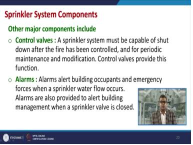
The other major component includes the control valves. The sprinkler system must be capable to shut down after the fire has been controlled and for periodic maintenance and modification. Control valves provide this function. Alarms, usually alarms alert building occupants and emergency forces. When a sprinkler water flow occurs, alarms are also provided to alert building management when a sprinkler valve is closed.
