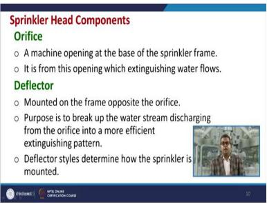
Now there is an Orifice, this is a machine opening at the base of the sprinkler frame and it is from the opening which is extinguishing the water flow so that the small droplets may appear and the excess amount of energy whatever being liberated during the course of fire may come out and may be trapped.
