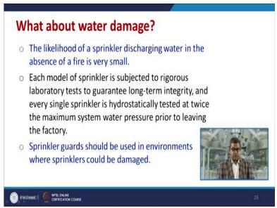
The likelihood of a sprinkler discharging water in the absence of a fire is very small, small amount of water. Each model of a sprinkler is subjected to rigorous laboratory test to guarantee the long-term integrity and every single sprinkler is hydrostatically tested at twice the maximum system water pressure prior to the leaving the factory or manufacturing facilities. A sprinkler guard should be used in environments where sprinkler could be damaged.
