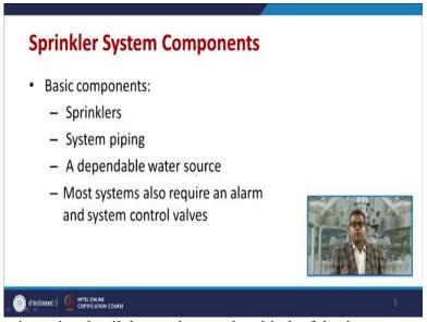
So before we go into the detail let us have what kind of basic components a particular sprinklers have. They are having the sprinklers, they are having the system piping, a dependable water supply or a water source and most systems also require an alarm and system control valves. So these are the four basic components which you require to install in sprinkler facility.
