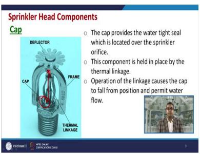
Then the cap, this one, the cap provides the water tight seal which is located over the sprinkler orifice. This one is the sprinkler orifice. Now this component is held in place by the thermal linkage, so operation of the linkage causes the cap to fall from the position and permits the water flow.
