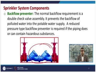
There are certain backflow preventers. The normal backflow requirement is a double check valve assembly, usually like this. It prevents the backflow of polluted water into potable water supply. So a reduced pressure type backflow preventer is required if the piping does or can contain hazardous substance. So sometimes it is the common problem in various chemical plants.
