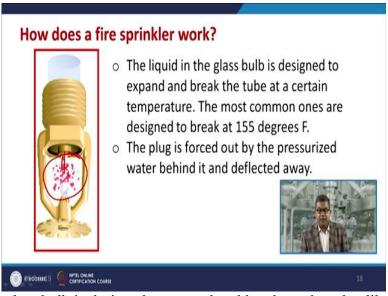
The liquid in the glass bulb is designed to expand and break up the tube, like this it is broken over here. They break the tube at a certain temperature, the temperature is specified or the most common ones are designed to break at 155 degree Fahrenheit. The plug is forced out by the pressurized water like this, here coming out pressurized water behind it and deflected away.
