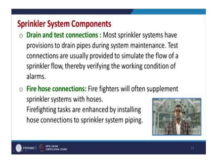
There are certain drain and test connections. Most sprinkler systems have provisions to drain pipe during the system maintenance. The test connections are usually provided to simulate the flow of a sprinkler flow, thereby verifying the working condition of alarms. There are certain fire hose connections. The fire fighters will often supplement a sprinkler system with hoses. The firefighting tasks are enhanced by installing hose connection to the sprinkler system piping.
