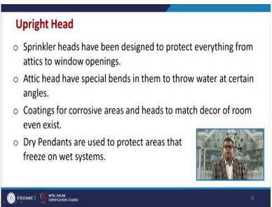
The upright head, the sprinkler head have been designed to protect everything from attics to the window opening. The attic head have special bend in them to throw the water at a certain angle. The coating for corrosive area and heads to match décor of a room even exist, that is the foremost requirement. Dry pendants are used to protect the areas that freeze on wet systems. So it is one of the remedy to avoid the freezing.
