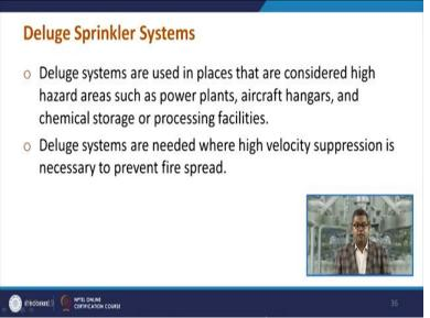
So the deluge systems are used in places that are considered high hazard areas such as power plant, aircraft hangars and chemical storage or processing facilities. So deluge systems are needed where high velocity suppression is necessary to prevent fire spread.
