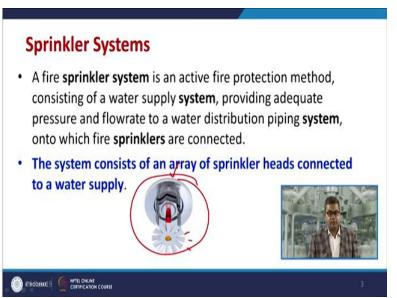
A fire sprinkler system is an active fire protection method consisting of a water supply system, providing adequate pressure and flow rate to a water distribution piping system, onto which fire sprinklers are connected. Now this system as you can see in this particular figure, this system consists of an array of sprinkler heads connected to a water supply. So we will discuss aspect in subsequent slide and we will discuss about the anatomy of a sprinkler head.
