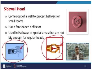
There are another type of sprinkler system, they are called a sidewall head and you can see in these figures, they are the sidewalls. Here, there is a side wall or a plate situated over there. They comes out of a wall to protect the Hallways or small rooms or you may put in the wall, so in case of any fire they can extinguish that particular fire, and has a fan shaped deflector like this and used in hallway or special area that are not big enough for the regular heads.
