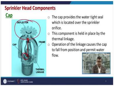
There is a deflector like this in the previous, this one is the deflector. Deflector mounted on the frame opposite to the orifice and the purpose is to break up the water stream discharging from the orifice into more efficient extinguishing pattern. And sometimes based on the requirement these deflectors are of different type. Now deflector style determine that how the sprinkler is mounted.
