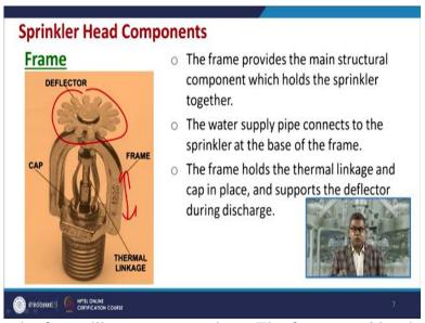
The first thing is the frame like you can see here. The frame provides the main structural component which holds the sprinkler together. The water supply pipe connect to the sprinkler at the base of the frame and the frame holds the thermal linkage, this one, and supports the deflector during the discharge so that, that can focus towards the problematic zone.
