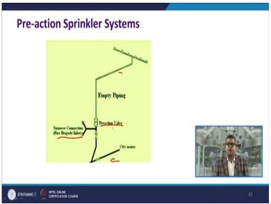
Now this is the figure which explains the preaction sprinkler system. There are the empty pipes and this is the preaction valve over here. There are fire brigade inlets etc, and this is the City mains. So this is a very small setup. Now in this particular module we have studied all kind of sprinkler system, what is the anatomy of the different sprinkler system; we have discussed all aspects, where to use and where not; advantages and disadvantages.
