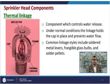
Now this one is a thermal linkage, this component which controls the water, releases. Under the normal condition the linkage holds the cap in place, this one is the cap in place, and prevents the water flow because these are the normal conditions. Now common linkages style include soldered metal lever, frangible glass bulb and solder pellets. Sometimes people may use wax and 70-80 years ago people were using the wax as a thermal linkage.
