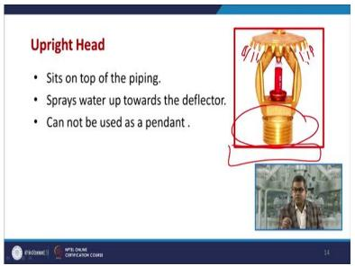
There are certain upright head type of sprinklers. They sit on the piping system and sprays water up towards the deflector like this and it cannot be used as a pendant, the reason is that the flow pattern is just reverse to the pendant type of sprinkler system.
