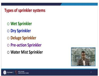
Now there are various type of sprinkler systems, like wet sprinkler, dry sprinkler, deluge type of sprinkler, pre-action sprinklers, water mist sprinklers and so on.
