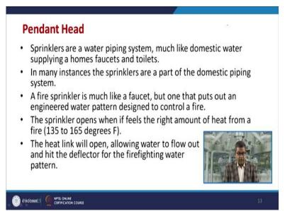
So sprinklers are the water piping system and much like domestic water supplying homes, faucet and toilets, etc. In many instances the sprinklers are part of the domestic piping system. A fire sprinkle is much like a faucet but one that puts out an engineered water pattern designed to control a fire. Because see, whenever you are having the excess water, then unnecessarily there would be a property damage, so you need to be, the sprinkler need to be focused in the problematic zone only.
