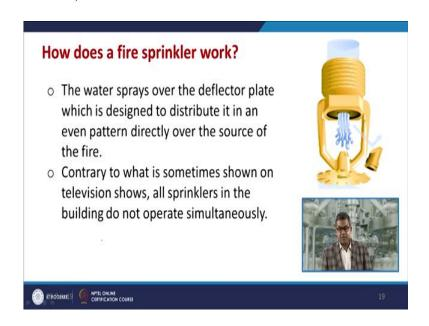
The water sprays over the deflector plate which is designed to distribute in an even pattern directly over the source of the fire. Contrary to what sometimes shown on the television, like shows, that all the sprinklers in the building do not operate simultaneously.
