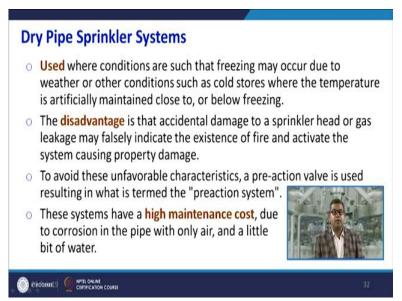
Now where to use this dry pipe sprinkler system? Used where the conditions are such that the freezing may occur due to the weather conditions, sometimes sub zero conditions etc, or other
