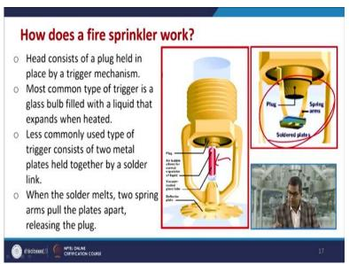
Now question arises, how does a fire sprinkler work? The head consist of a plug held in place of a trigger mechanism. And most common type of trigger is a glass bulb filled with a liquid that expands when heated. So less commonly used type of trigger consists of two metal plates held together by a solder link so that the difference in the temperature can actuate the
