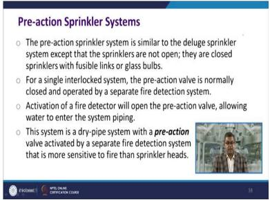
Now the last segment in this category is the preaction sprinkler system. The preaction sprinkler system is similar to the deluge sprinkler system, except that the sprinklers are not open; they are closed sprinklers with fusible link or glass bulbs. For a single interlocked system, the preaction valve is normally closed and operated by a separate fire detection system.
