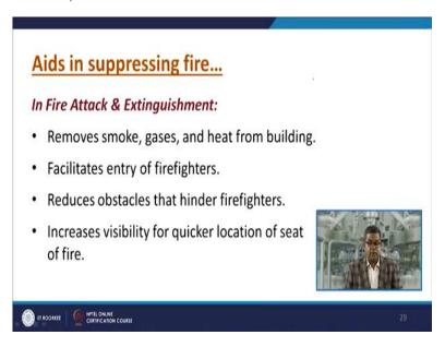
Now aids in suppressing fire in fire attack or extinguishment removes smoke, gases and heat from building. Facilitates entry of firefighters because the visibility is on the higher side. Reduces the obstacles that hinder the firefighters. Increases visibility for quicker location of seat of fire.
