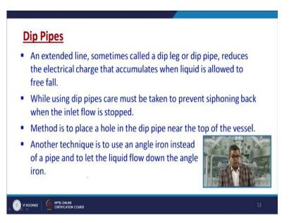
Now, another aspect is that dip pipe. Usually this is an extended line or sometimes called a dip leg or dip pipe which reduces the electric charge that accumulates when liquid is allowed to free fall. While using dip pipe care must be taken to prevent the siphoning back when the inlet flow is stopped. The method is to place a hole in the dip pipe near the top of the vessel. Another technique is to use an angle iron instead of a dip pipe and let the liquid flow down to an angle iron.
