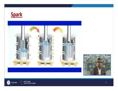
Now there is another possibility of spark or spark charge transfer. This is the vessel filling operation, now there are three aspects, one is this one, another one is that the outer periphery you may generate the charge and third one is that how we can reduce the impact of this generation of spark. So, this figure, particular figure depicts that how we can minimize this charge transfer and how we can minimize the effect of spark generation.
