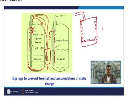
Now here it is the best example that how dip legs prevent the free fall and accumulation of static charges. So before we discuss this one let us have what happened at the start-up. Suppose I am having this vessel to be filled with flammable liquid and one option is that I am flowing
