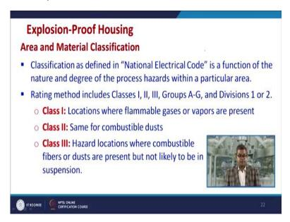
Now, how we can classify this explosion proof housing? This slide will discuss the classification are usually defined on the basis of national electrical code that is based on United States federal law and this is a function of nature and degree of the process hazards within a particular area.
