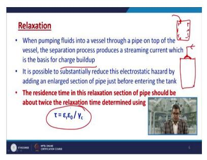
Now relaxation. Sometimes relaxation because the charge density is a very crucial point, so relaxation is one of the most effective or you can say the effective tool to minimize the effect of electrostatic ignition. So, when you are pumping fluids into a vessel through a pipe on the top of the vessel, like this, the separation process produces a streaming current, like this, which is the basis of charge build up.
