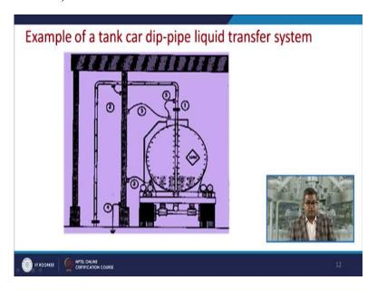
This is again, the best example of streaming charge effect. Now this particular lorry contains a flammable liquid. Let us have some practical example of petrol or motor spirit, this lorry carries the motor spirit so during the transit or during the transportation from the depot to the petrol pump, it may have certain accumulated charges, either at the inner part like this at the surface or over the fluid surface.
