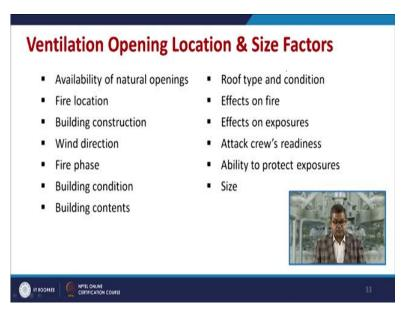
Now ventilation opening location and size factors they depend on the availability of natural opening because obviously for this opening you need not to pay any penny. Fire location, what is the fire location. Building construction of what type. What is the wind direction although it is not constant throughout. Fire phase, building Condition, what is the building condition,
