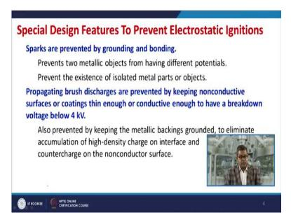
Now, there are certain special design features for the prevention of electrostatic ignition. Sparks usually they are prevented by grounding and bonding so grounding and bonding they are very useful and common phenomenon for elimination of the hazard of electrostatic ignition. Now, they prevent two metallic objects from having the different potential, prevent the existence of isolated metal parts or objects.
