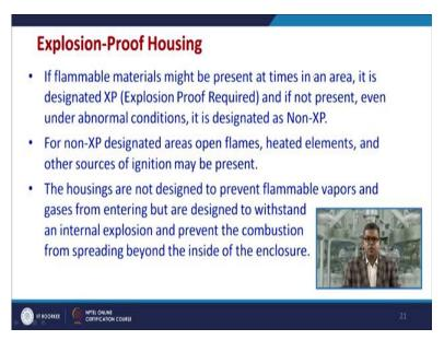
Now, if flammable materials might be present at time in an area, it is designated XP that is explosion proof required and if not present even under abnormal condition it is designated as non-explosion proof required area, so that means you can avoid the installation of such safety devices. So, for non-explosion proof required designated area open flames, heated elements and other sources of ignition may be present because you can work it upon.
