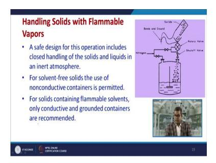
Sometimes you may need to handle another scenario where you cannot perform this type of activity which we have discussed in the previous slide. Then you need to adopt the concept of inerting. Now here you are handling with the flammable vapours so when your continuously filling solids to this particular reactor, this is a solid liquid reaction so in that particular case the chances of generation of charge are on the higher side and sometimes you may not be in a position to ground it properly.
