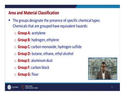
Now the groups, they are designated to presence of specific chemical type and the chemicals that are grouped have equivalent hazards like Group A acetylene or equivalent; Group B hydrogen, ethylene; Group C carbon monoxide, hydrogen sulphide, Group D butane, ethane, ethyl alcohol, Group E aluminium dust, Group F carbon black, Group G flour.
