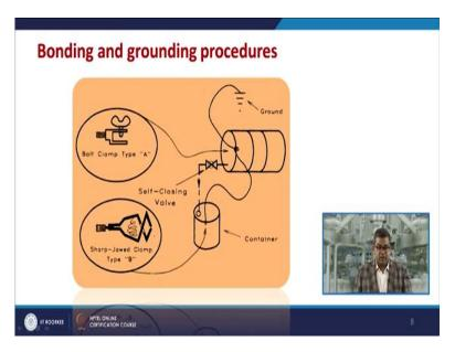
Now this is the pictorial explanation of this bonding and grounding. Now here, we have a container which is duly grounded. Now this is the container and these two, these Bolt clamp, type A and type B both are joined together, and this is the best example of bonding and grounding.
