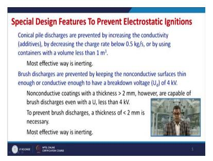
Conical pile discharges they are prevented by increasing the conductivity, by addition of certain additives, we will discuss in due course of time, by decreasing the chare rate below around they say 0.5 kilogram per second or by using the containers with volume less than 1 meter cube. Now the most effective, remember the most effective way is inerting. So, if your inerting is efficient then definitely you can avoid the hazard of electrostatic ignition.
