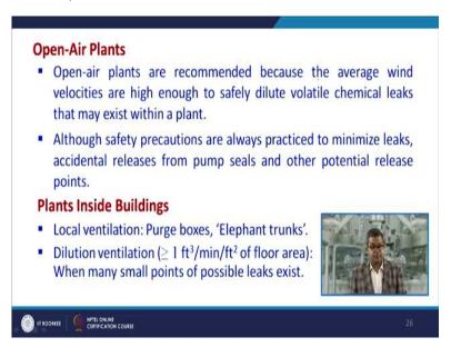
There are certain open-air plants so open-air plants are recommended because the average wind velocities are high enough to safely dilute the volatile chemical leaks if any and that may exist within a plant. Sometimes it may create a problem of unconfined vapour cloud explosion. So,
