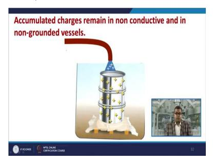
Now this is again a very common phenomenon that is accumulated charge remain in non-conductive and non-grounded vessel. If your filling any vessel with any fluid, if it is not properly been grounded or bonded then the charge will remain to the surface of this particular vessel and whenever this particular vessel will come into contact to certain favourable conditions then spark may generated. So be careful and adopt the concept of grounding.
