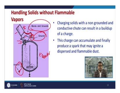
Sometimes you need to encounter the problem of handling solid without flammable vapours so here again you need to adopt the proper bonding and grounding aspect like here you can see, these two are bonded each other. Now here before we go into detail, this particular solid is being filled with this funnel to this particular reactor so while transferring this solid material through this hopper or a funnel to this reactor there may be a chance of generation of static charge.
