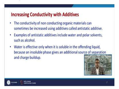
Another methodology is to increase the conductivity by the addition of additives. So, the conductivity of non-conducting organic materials can sometimes be increased using the additives, they are called the antistatic additives. Examples of antistatic additives include water and polar solvents such as alcohol, etc. Water is effective only when it is soluble in the offending liquid because an insoluble phase gives an additional source of separation and charge build up.
