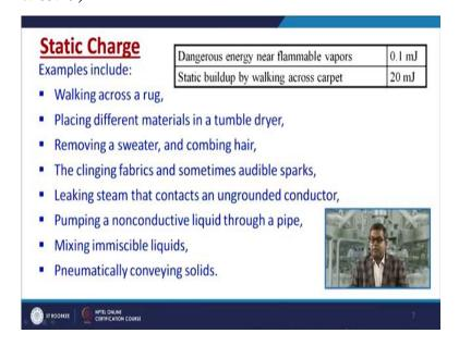
Now, you may have look that a dangerous energy near the flammable vapours is around 0.1 milli Joule. And if you walk across the carpet or you are simply walking across the floor then the generation of static charge is around 20 milli Joule. So, you can anticipate that how dangerous it is. So, it is the foremost requirement to remove whatever excess charge or static charge build up on the surface to avoid any kind of fire and explosion hazard.
