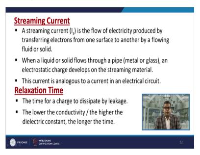
Another concept is the streaming current, especially when you are transferring an inflammable material from one place to another place, the concept of stream current plays a very vital role, so a streaming current is the flow of electricity produced by transferring electrons from one surface to another by flowing fluid or solid especially valuable when you are transferring hydrocarbon from one place to another place.
