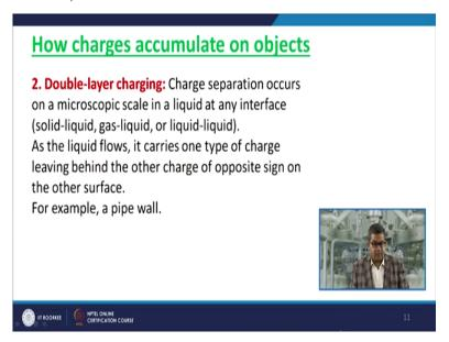
Second is the double layer charging. Charge separation occurs on a microscopic scale in a liquid at any interface maybe solid-liquid, gas-liquid or liquid-liquid. So, as the liquid flows, it carries one type of charge leaving behind the other charge of opposite sign on the other surface. The best example is a pipe wall.
