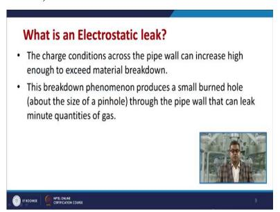
Now, sometimes we may experience the electrostatic leak. So, question arises that what is an electrostatic leak? The charge conditions across the pipe wall can increase high enough to exceed material breakdown. And this breakdown phenomenon produces a small burned hole about a size of a pinhole through a pipe wall that can leak the minute quantities of gases.
