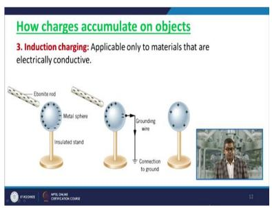
The third one is the induction charging. This is applicable only to the material that are electrically conductive. So, you can see that you are having one metal sphere over here. This is the insulated stand, and this is the Ebonite rod. So, the charge accumulation takes place in
