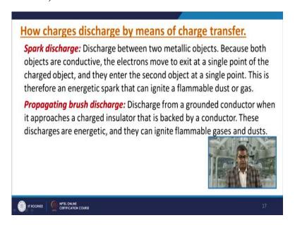
There is another aspect that is called the spark discharge that is the discharge between to metallic objects because both objects are conductive, the electrons move to exit at a single point of the charged object and they enter the second object at a single point and this is therefore an energetic spark that can ignite a flammable dust or a gas.
