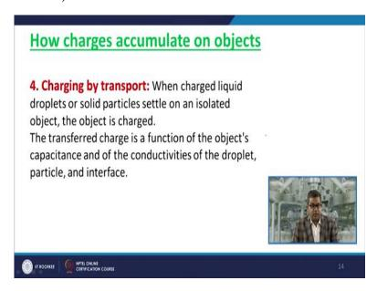
The last part is that charging by transport so when charged liquid droplets or solid particles settle on an isolated object the object is charged. The transferred charge is a function of the object's capacitance and of the conductivities of the droplet, particle and interfaces. So, this is again a very useful phenomenon and very common phenomenon in chemical engineering aspect.
