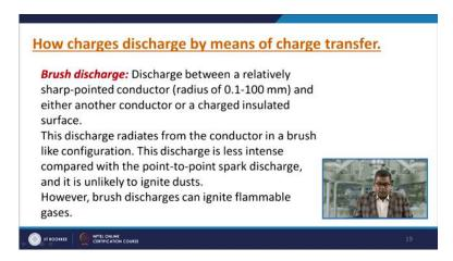
Now brush discharge, the discharge between a relatively sharp-pointed conductor usually the radius of about 0.1 to 100 millimetre and either another conductor or charged insulated surface. This discharge radiates from the conductor in a brush like configuration and this discharge is less intense compared with the point to point spark discharge and it is unlikely to ignite dusts. However, brush discharge can ignite flammable gases, so the gravity is on the higher side.
