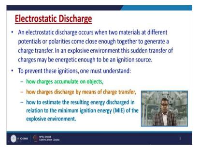
So, electrostatic discharge is usually an electrostatic discharge occurs when two materials at different potential or polarities come close enough together to generate a charge transfer. In an explosive environment this sudden transfer of charge maybe so energetic to be a source of ignition. So, remember we must aware this type of danger, because these are certain hidden dangers in our work place.
