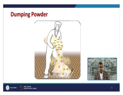
Sometimes this type of a problem when you are dumping the powder or bags to storage area or anywhere else then you may experience this type of problem, the negative charge particle and the positive charge particle so you have to take the due care while handling such type of scenario.
