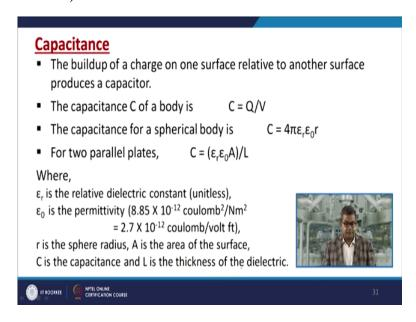
Let us have a discussion about the capacitance that is the buildup of charge on surface related to another surface produces a capacitor. The capacitance C of a body is denoted by:
