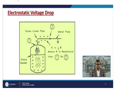
Now, this is again the electrostatic sometimes the electrostatic voltage drop may create a problem especially when you are adopting the concept of vessel filling operation. Now, this is the glass lined pipe with a certain fluid is flowing through this glass line pipe and this pipe is connected to this vessel where this vessel is being filled by this particular pipe.
