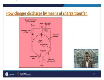
So, in this particular figure you can see that this is a typical filling operation when the solids are being filled in a vessel and they are passed through the hoppers because solid particles they by the friction or the by the transfer they may charge, they may generate the static electricity or static charge so this particular vessel is properly grounded like this, this grounded thermo wall to all metals.
