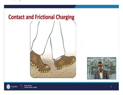
This is a very common aspect that is contact and frictional charging so you are moving across any surface, may be floor, may be carpet, may be grass, etc based on the material of your sole the charge may accumulate or charge may generate so when they find the favourable condition the spark may be created and that is why and if the chances are on the higher side when your shoe is equipped with iron shoe nails so be practical and be aware about such particular scenario.
