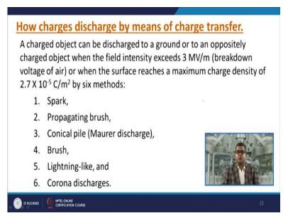
Now, another question is how charge is discharged by means of charge transfer? So, a charge can be discharged to a ground or to an oppositely charge object when the field intensity exceed by 3 mega volt per meter, breakdown voltage of air or when the surface reaches the maximum charge density by different six methods. So, there are six methods through which it reaches the
