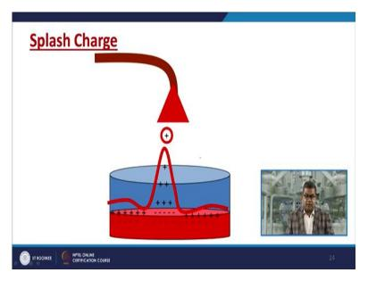
Another is the splash charge, especially it is applicable in the vessel filling application so you are filling a vessel and the discharge point or the outlet of this pipe is at this point so whenever
