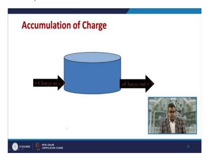
Sometimes the accumulation of charge may take place in static vessel where the charge in and the charge out may be in the neutral side so sometimes you may experience the accumulation of charge within the vessel without the reason unknown and sometimes it may pass on to some other surface.
