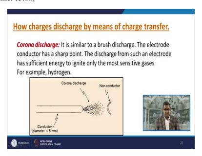
The Corona discharge, it is similar to the brush discharge. The electrode conductor has a sharp point. The discharge from such an electrode has sufficient energy to ignite only the most sensitive gases like Hydrogen so here you can see the accumulation of charges, so this is a non-conductor.
