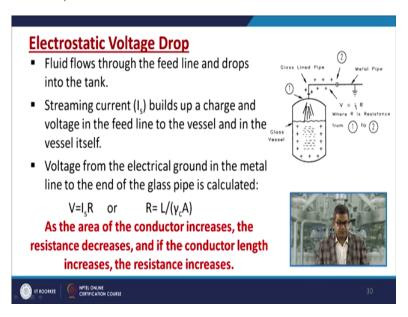
So, fluid flows through the feed line and drops into the tank and streaming current that is represented by Is builds up the charge and voltage in the feed line to the vessel and in the vessel itself. So, voltage from the electrical ground in the metal line to the end of the glass pipe is calculated through this formula:
