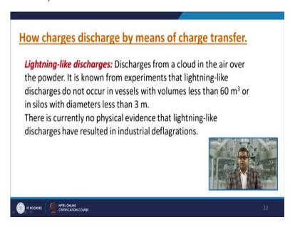
Another method is lightning like discharges that is discharge from a cloud in the air over the powder. It is known from the experiments like lightning-like discharge do not occur in vessel with volume less than 60 meter cube or in silos where diameter is less than 3 meters. There is currently no physical evidence that lightning like discharges have resulted in industrial deflagrations.
