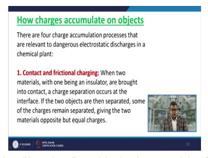
So, in the previous slides we have discussed that there is an accumulation of charges on an object. So, question arises that how charges are accumulate on an object. So there four charge accumulation processes that are relevant to the dangerous electrostatic discharge in a chemical plant. Number 1, the Contact and frictional charging. So, when two materials with one being an insulator are brought into contact, a charge separation occurs at the interface. If the two
