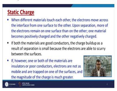
Now, let us discuss about the static charge. So, when different material touch each other, the electron moves across the interface from one surface to other. Upon separation, more of the electrons remain on one surface than on the other. So, one material becomes positively charged and other negatively charged. Now, if both materials are good conductor the charge build up as a result of separation is small because electrons are able to scurry between the surface.
