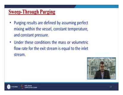
Now, purging results are defined by assuming perfect mixing within the vessel. Constant temperature and a constant pressure. So, under these conditions the mass or a volumetric flow rate for the exit stream is equal to the inlet stream. So, these are certain things we need to keep in mind.
