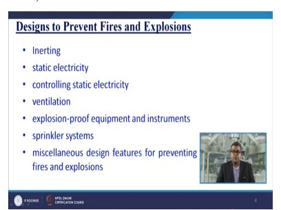
Now, question arises that how we can design the system? So there are seven broad spectrums through which we can go ahead with designing aspect. Inerting, static electricity, controlling static electricity, ventilation, explosion-proof equipment and instruments, sprinkler system and miscellaneous design features for preventing the reference. So we will discuss all the aspect in due course of time in various models.
