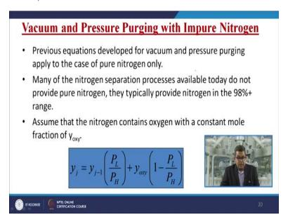
Sometimes we may have to use the vacuum and a pressure purging with impure Nitrogen. So, previous equation which we have discussed, developed for the vacuum and pressure purging apply to the case of pure nitrogen only. Many of the Nitrogen separation processes available today do not provide pure Nitrogen they typically provide the Nitrogen in the range of 98 percent plus minus range.
