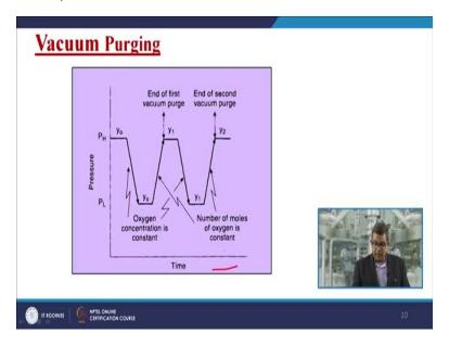
We can understand this particular aspect with this small plot here at the x-axis we are having the time domain and at y-axis the pressure domain.
