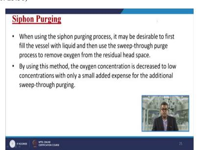
So, when using the siphon purging process it may be desirable to first fill the vessel with the liquid then use sweep-through purging process to remove oxygen from residual head space. Now, by using this method the oxygen concentration is decreased to low concentration with only a small added expense for the additional sweep-through purging. So, these things should be in our mind.
