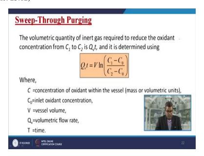
Now, here is one of the mathematical relations through which you can analyze the volumetric flow rate. The volumetric quantity of inert gas require to reduce the oxidant concentration from  $C_1$  to  $C_2$ , let us have  $Q_v t$  and it is determined using this particular equation:
