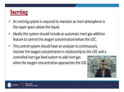
An inerting system is required to maintain an inert atmosphere in the vapor space above the liquid. Suppose, I am working here in a pool of say hexane and just because of its vapor pressure certain quantity of vapors has been generated and just above the pool of liquid surface. So, by virtue of my system design I am not in a position to cordon off oxygen or supply of air. Then inerting is a useful way (to inert) to minimize the impact of fire hazard.
