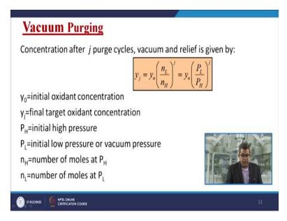
Now this is, you can calculate this through small mathematical formula that is concentration after J purge cycles suppose in the previous case we have to studied 2 purge cycles, concentration after J purge cycles vacuum and relief is given by:
