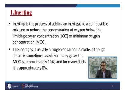
So, let us have first thing that is Inerting. Inerting is a process of adding an inert gas to a combustible mixture to reduce the concentration of oxygen below the limiting oxygen
