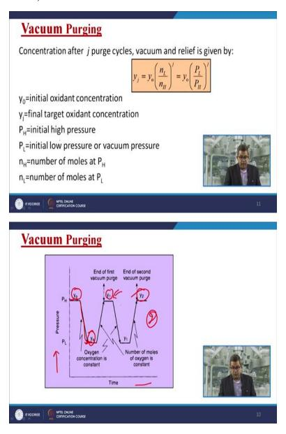
Now here the  $P_H$  is the initial high pressure this one and  $P_L$  is the initial low pressure or desired vacuum pressure.  $Y_0$  is initial oxidant concentration and  $Y_1$  is the final target oxidant concentration, so first thing is that you are having certain quantity of oxygen in a system specially suppose you are willing to have an introduction of inert gas to a vessel. Then initially you are having  $Y_0$  concentration of Oxygen.
