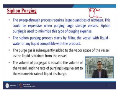
Another purging method is the Siphon purging. Now sweep-through purging process requires large quantity of nitrogen. Because you need to fill the entire mass of I mean entire volume of the vessel with the nitrogen. Now, this could be expensive when purging a large storage vessel. So, Siphon purging is used to minimize this type of purging expenses. Now, it is a very simple and quite
