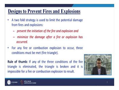
Now, first of all let us have a discussion about how to prevent the fire and explosion. Usually a twofold strategy is used to limit the potential damage from fires and explosion. One is the prevent the initiation of fire and explosion obviously this is one of the foremost requirement and the second is that minimize the damage after a fire or explosion has occurred. For any fire or combustion explosion to occur, three conditions must be met.
