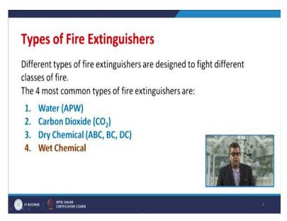
Now, we have discussed different type of Fire Extinguishers so until now we have discussed about the Air Pressurized Water Fire Extinguisher, Carbon Dioxide based Fire Extinguishers, Dry chemical based Fire Extinguishers.
