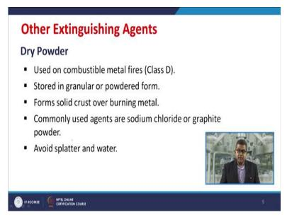
There are certain Dry powders being used as fire extinguishment media. Now they used on the combustible metal fires that is attributed to Class "D" fire. Usually they are stored in granular or powdered form and this forms solid crust over the burning material so it can cordon off the fuel supply with the atmospheric Oxygen, so it creates the blanket and that is why the fire is extinguished. Commonly used as agent as Sodium Chloride or a Graphite powder, avoid splatter and water.
