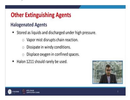
Usually it is stored as liquid and discharged under very high pressure. Now, vapor mist disrupts chain reaction, this is one of the added benefits of Halogenated agents. Dissipate in windy condition and Displace Oxygen in a confined space so these are some of the added benefits of these Halogenated agents. One advisory is that the Halon 1211 should rarely be used because it creates the environmental problem.
