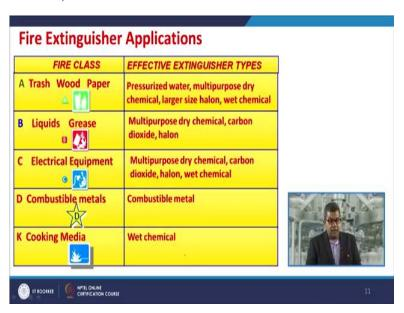
Now, in a nutshell you can see in this particular slide that different class of fire and effective extinguisher types. That means you can have a look, or you can have a idea that what are the different applications of these fire extinguishers. So, class "A", trash wood paper, usually pressurized water, multipurpose dry chemical being used, larger size Halons and wet chemicals.
