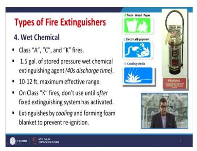
Now, in this particular module we will start with Wet Chemical Fire Extinguishers. Now, this Wet Chemical based Fire Extinguisher is applicable for Class "A", Class "C" and Class "K" of fire. This is one of the kind of Wet Chemical Fire Extinguisher. Usually they are having 10 to 12 feet effective range, so you must know that from where or how proximity you have to use this Fire Extinguisher.
