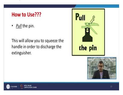
Now, first thing is that how to use it? That is the pull the pin, as I showed you in the anatomy of a fire extinguisher there is a pin. So, you need to pull that pin out. This will allow you to squeeze the handle, these handles, in order to discharge the extinguishing media towards the fire.
