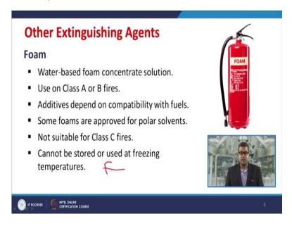
Foam, usually this is another class of fire extinguishing agent and it is one of the most common type of fire extinguishment media that is foam. This is the water based foam, concentrate solution used on Class "A" or Class "B" type of fire. Sometimes we may use different additives, so additive depend on the compatibility with the fuel that is the next source of fuel.
