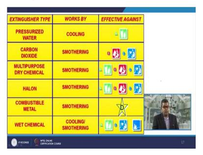
So, you can again have a look different type of extinguisher, then works by, then effective agents which you can use that pressurized water, it works by cooling, Carbon dioxide smothering, multipurpose dry chemical is smothering, Halon based smothering, combustible metals they again smothering and the wet chemicals cooling and smothering so different types of effective agents.
