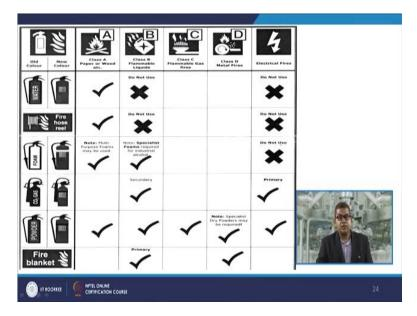
Now, again this type of chart or this type of play card should be placed at appropriate place that what kind of fire extinguisher available at your place, what kind of fire or what class of fire, you can use that particular fire extinguisher and it should be properly mentioned that do not use this type of fire extinguisher in such a class of fire.
