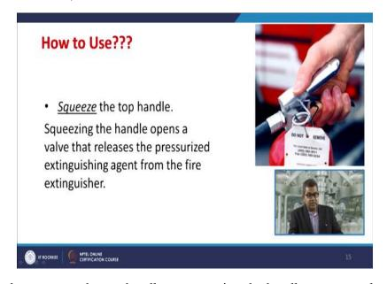
Then you need to squeeze the top handle so squeezing the handle opens a valve that releases the pressurized extinguishing agent from the fire extinguisher. So, this type of advisories always put on the fire extinguisher.
