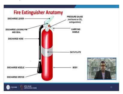
Now, this is the Fire Extinguisher anatomy. You can think upon the basic methodology and basic anatomy of this Fire Extinguisher, they are having the discharge liver, so you can press it with the help of this carrying handle to release the pins, the pin they are located over here, that is a Discharge locking pin and seal so that accidentally if anybody presses then definitely it will come out.
