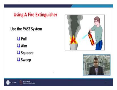
Now, how to use the fire extinguisher? Usually we may follow the PASS system. Now PASS system says Pull, aim towards the fire, Squeeze means you just put the liver and sweep away like this. So, your industrial workers, etc must be trained for this type of PASS system.
