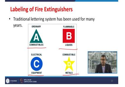
Now traditional lettering system has been used for many years that is for the labeling of fire extinguishers like ordinary class A ordinary combustible, flammable liquids class B, electrical equipment C and combustible metals D, these are the traditional one.
