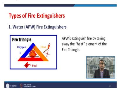
Now APWs they extinguish fire by taking away the heat element of the fire triangle because of the formation of small droplets.
