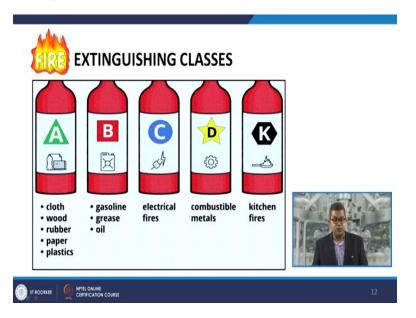
So you may see different type fire extinguishers in different places you visit or different industry you work upon, so there are different classes of fire extinguishers: one is the class A basically attributed to cloth, wood, rubber, paper, plastic; class B gasoline, grease, oil; class C, electrical fires; class D combustible metals; class K that is the kitchen fires etc.
