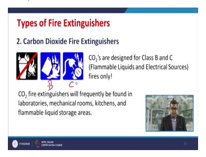
Now CO<sub>2</sub> are designed for class B and class C type of fires, flammable liquid and electrical sources fire. CO<sub>2</sub> fire extinguishers will frequently be found in laboratories, mechanical rooms,
