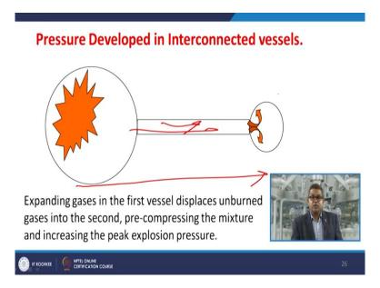
Now how it can happen? Now this is again the 2 scenario, they are interconnected, this device and certain quantity of dust is being accumulated over here. So expanding gases in the first vessel they displace unburned gases into the second one from here and pre-compressing the mixture and increasing the peak explosion pressure because they are well interconnected. So by this way there may be a chance that the dust or pressure whatever is accumulated being exploded.
