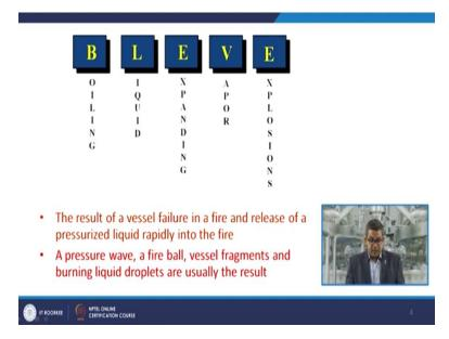
Now BLEVE, the boiling liquid expanding vapor explosion, this is extremely dangerous and destructive explosion. Now the result of vessel failure in a fire releases a pressurized liquid rapidly into fire, now a pressure wave is being generated, a fire ball is being created and the vessel fragments and burning liquid droplets are usually formed in terms of a result.
