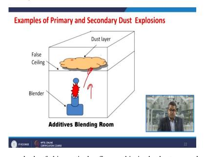
Now you can have a look of this particular figure, this is the best example of primary and secondary dust explosion. It have a blender, the additive blending room; this particular room is equipped with the false ceiling and there is a small quantum of dusty layer. This is accumulated over the period of time, now this while working this blender with this blender a certain quantity of fine particles is being generated.
