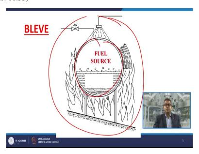
Now this is the typical figure of BLEVE, here this the fuel source and it is surrounded this entire vessel is being heated by some other sources.
