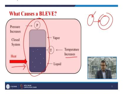
Now it is you can visualize the things through this figure, suppose we are working in a particular closed system and pressure increases and somehow it catches the heat just like in Jaipur one vessel caught the fire and heat propagated to the another vessel and this is being heated up. So by any means it catches the heat and the liquid though somehow temperature rises or temperature increases and the formation of vapors propagated.
