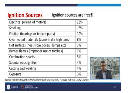
We have collected some statistical information about the ignition sources, this is based on the accidental investigation, so electrical motor or wiring of motor they causes almost 23 percent of accident; smocking 18 percent; friction bearing or broken parts, almost 10 percent; overheated
