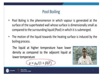
So, pool boiling usually is a phenomenon in which vapour is generated at the surface of a superheated wall whose surface is dimensionally small as compared to the surrounding liquid that is a pool in which it is submerged. So, the motion of the liquid towards the heating surface is induced by the boiling process. Now, the liquid at higher temperature have the lower density compare to the adjacent liquid at the lower temperature.
