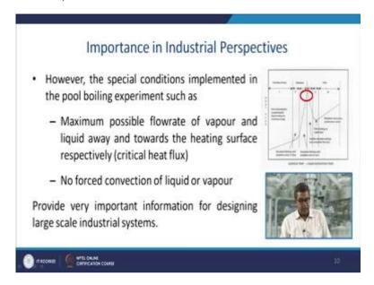
Now, however the special conditions usually implemented in the pool boiling experiments such as a maximum possible flow rate of vapour and a liquid away and towards the heating surface respectively that is called the critical heat flux and the no forced convection of liquid or vapour. So, provided very (impor) this provides a very important formation for designing the large scale industrial system.
