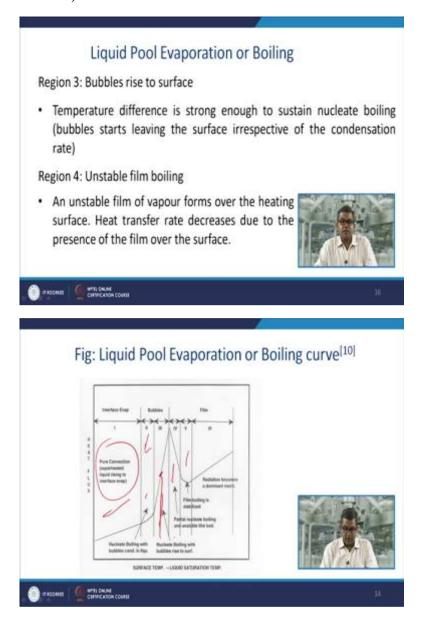
In the third region, that is bubble rise to the surface, this one, the bubbles rise to the surface. The temperature difference is a strong enough to sustain Nucleate boiling, bubbles start leaving the surface irrespective of the condensation rate. Now, in the fourth region, this one is the fourth region, now that is a unstable film boiling, the unstable film of vapour forms over the heating surface and a heat transfer rate decrease due to the presence of film over the surface.
