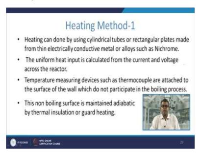
So, let us have different heating methods. So, in method number one, the heating can be done (use) using cylindrical tubes or rectangular plate mould made from thin electrically conductive material or metal or (allow) alloys such as Nichrome. The uniform heat input is calculated from the current and voltage across the reactor. The temperature measuring devices such as thermocouple are attached to the surface of the wall which is which do not participate in the boiling process.
