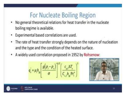
Now, let us have a look of the Nucleate boiling reason. There is no general theoretical relations for heat transfer in the Nucleate boiling regime. Experimental based correlations are sometimes used. The rate of heat transfer strongly depend on the nature of nucleation and the type and the condition of the heated surface.
