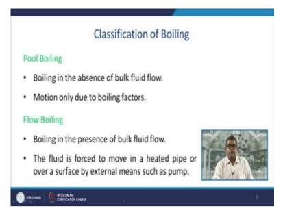
So, whenever we are considering the boiling, boiling is divided in two different categories like pool boiling, flow boiling. So, pool boiling, boiling, this is the boiling in the absence of bulk fluid flow where and motion only due to the boiling factors, so these are the this is related to the pool boiling. And we consider the flow boiling, the boiling is in the presence of bulk fluid flow and the fluid is forced to move in a heated pipe or over a surface by external means such as pump.
