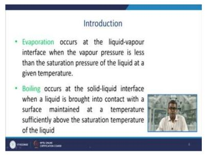
So, evaporation occurs at the liquid vapour interface when the vapour pressure is less than the saturation pressure of the liquid at a given temperature. Whereas boiling, this occurs at the solid-liquid interface when a liquid is brought into contact with a surface mentioned at a temperature sufficiently above the saturation temperature of the liquid. So, this is the basic difference between the evaporation and a boiling.
