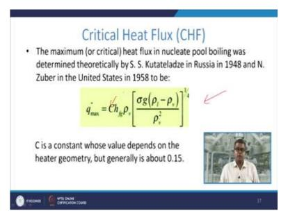
The critical heat flux, the maximum or critical heat flux in nucleate boiling was determined theoretically by S. S. Kutateladze in Russia in way back in 1948 and N. Zuber in the US in 1958. So, it is a represented by this particular equation,
