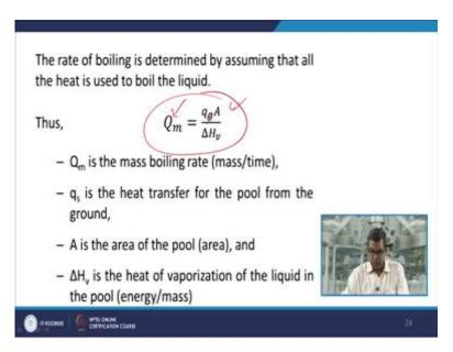
So, the rate of boiling is determined by assuming that all the heat is used to boil the liquid, that is thus, so
