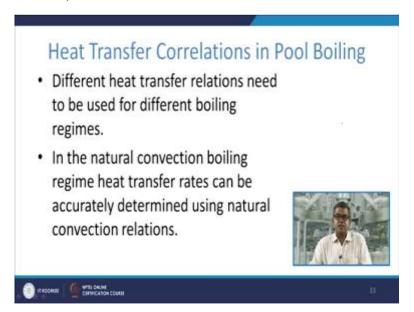
Now, let us have a look of heat transfer correlation in pool boiling. Now, different heat transfer relations need to be used for different boiling regimes. In the natural convection boiling regime heat transfer rates can be accurately determined using the natural convection relations.
