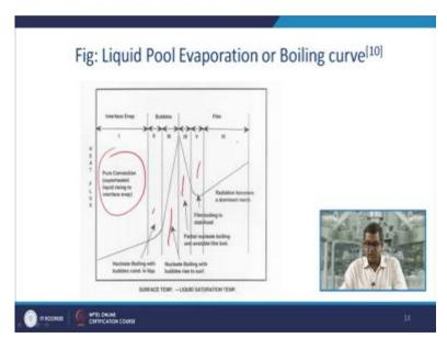
Now, this curve can be divided into six regions, which is represented here, region one, there the pure convection, superheated liquid rising to the interface, this is the Nucleate boiling with
