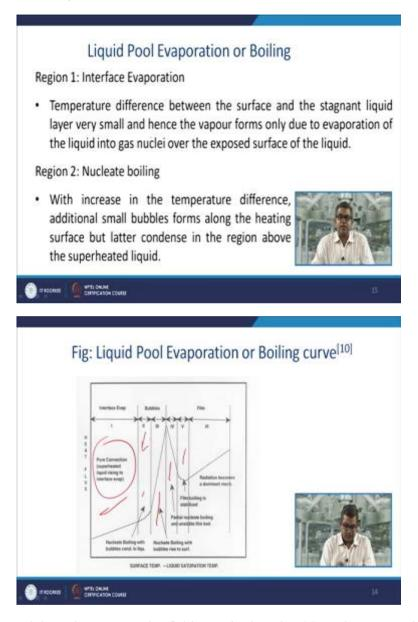
So let us have an elaborative approach of this particular plot. Now, let us consider this region one, this region one temperature difference between the surface and the stagnant liquid layer, very small, hence the vapour form only due to the evaporation of the liquid into gas nuclei over the exposed surface of the liquid, you can have a look of this particular region. Now, second region that is the Nucleate boiling this one.
