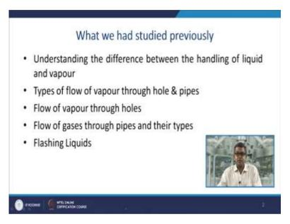
We have gone through the difference between the handling of liquid and vapours. We have discussed various types of flow of vapour through hole and pipe and the model and we discuss the various models. Flow of vapours through holes we have discussed about a flow of gases through pipes and their types. We have gone through the flashing of liquids.
