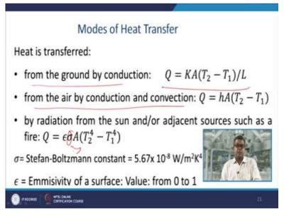
So, different modes of heat transfer while considering if this aspect then heat is transferred from the ground by the convection usual equation applicable is
