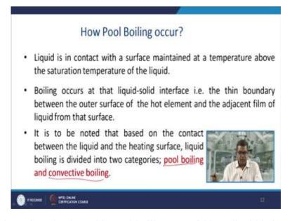
So, usual question arises that how this pool boiling occur? Now, liquid is in contact with the surface maintained at a temperature above the saturation temperature of the liquid, so boiling occurs at the liquid solid interface that is the thin boundary between the outer surface of the hot element and the adjacent film of liquid from the surface. Now, one thing to be noted that based
