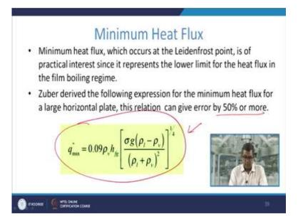
The minimum heat flux, the minimum heat flux, which occurs at the Leidenfrost point, is of the practical interest since it represents the lower limit of heat flux in the film boiling region. Now, Zuber derived this particular expression for the minimum heat flux for a large horizontal plate and this relation can be given by 50 percent or more.
