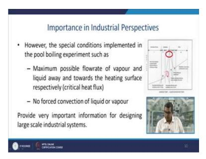
Now, the peak heat flux or burnout heat flux represents the upper limit of fully developed Nucleate boiling, you can have a look in this particular, this is a Nucleate (boiled) boiling zone, this one. So, while designing the engineering component, this heat flux provides the maximum limit of safe operation beyond this limit heat removal rate from the surface of heating device degrade substantially and this lead the melting or burnout of the surface.
