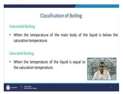
Another aspect is, the subcooled boiling, so usually occurs when a temperature of main body of the liquid is below the saturation temperature. Saturated boiling, when the temperature of
