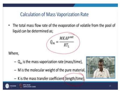
Now, for this the calculation of mass vaporization rate is carried out, so the total mass flow rate of evaporation of a volatile from the pool of a liquid, this is determined by this equation, earlier in different module we have derived this particular equation,
