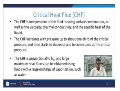
Now, this CHF that is the critical heat flux is independent of the fluid heating surface combination as well as the viscosity, thermal conductivity and the specific heat of the liquid. The CHF increases with the pressure up to about one-third of the critical pressure and then starts to decrease and becomes zero at the critical pressure. The CHF is proportional to  $h_{fg}$  and a large maximum heat fluxes can be obtained using the fluid with the large enthalpy of vaporization such as water.
