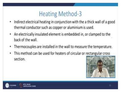
The third method is, the indirect electrical heating in conjunction with the, with the a thick wall of a good thermal conductor such as copper or aluminium. An electrically insulated element is embedded or clamped to the back of the wall. The thermocouples are installed in the wall to measure the temperature. Now, this method can be used for heater of circular or rectangular cross section.
