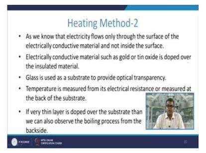
Another method attributed, now as we know that electricity flows only through the surface of electrically conductive material and not inside the surface. So, electrically conductive material such as gold or tin oxide is doped over the insulated material. Glass is used as a substrate to provide the optical transparency. Now, temperature is measured from its electrical resistance or measured at the back of the substrate.
