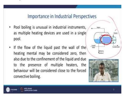
There are certain important industrial perspectives, now pool boiling is unusual in industrial instruments as multiple heating devices are used in single pool. Now, if a flow of liquid past the wall of the heating mental may be considered zero, then also due to the confinement of the
