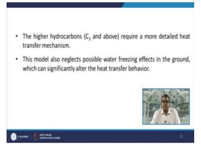
The higher hydrocarbons especially from C3 and above require a more detail heat transfer mechanism. Now, this model also neglects the possible water freezing effect in the ground and which can significantly alter the heat transfer behavior, this is very important phenomenon.
