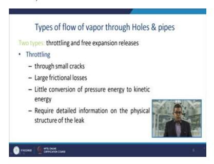
Now, let us have a look about the types of flow of vapour through holes and pipe. Now, there are two type of things, one is throttling and other one is the free expansion release. Now, throttling we all know may be through a small cracks, there is a large frictional losses, a little conversion of pressure energy to kinetic energy, they require the detailed information on the physical structure of the leaf.
