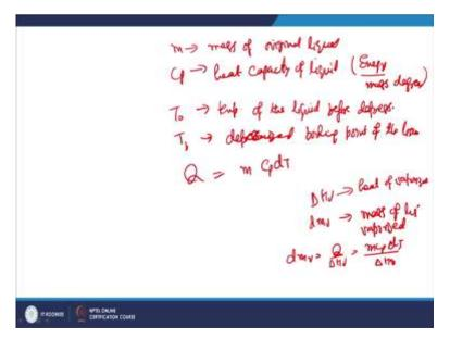
Now, if m is the mass of a original liquid, mass of original liquid and  $C_P$  is the heat capacity of the liquid energy plus mass degree and  $T_0$  is the temperature of the liquid before (depressive) depressurization, temperature of the liquid before the depressurization,  $T_b$  is the depressurized boiling point of the liquid. So, excess energy contained the superheated liquid may be calculated by this original thermodynamic equation,
