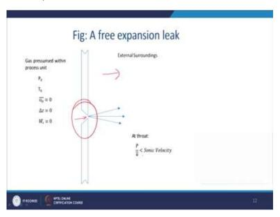
Now, let us have a look about a free expansion leak. Now, here we can visualize this figure you are having a gas pressurized within a process unit and it leaks through this particular point. So, initial condition if we say that  $P_0$ ,  $T_0$ ,  $u_0$  is equal to 0,  $\Delta z$  is equal to 0 and shaft work is equal to 0 and here the things are at the external surrounding. So, here you can have a throat where P is
