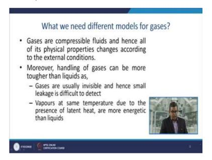
Now, what we need in different models for gases. Now, usually gases are compressible fluids and hence all of its physical properties changes according to the external conditions, these external conditions may be pressure, may be temperature, etcetera. Moreover handling of gases can more tougher than liquid. Now, because of the variety of reasons because one reason is,
