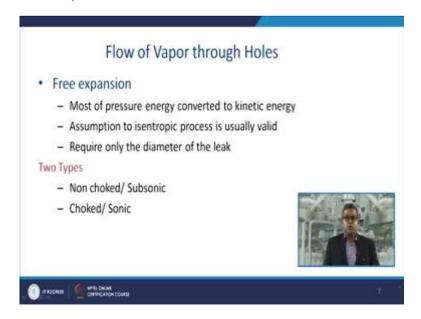
Whereas in a free expansion, the most of the pressure energy converted into kinetic energy, assumptions to isentropic process is usually valid because while you consider this free expansion you may have to take certain assumptions. So, one assumption is to the isentropic process which is usually valid in this case. Now, they require only a diameter of a leak, so this is a bit easier.
