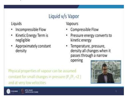
Now, here we have a comparison of liquid versus vapour, liquid usually they are compressible flow whereas vapours they are the compressible one. In liquids, the kinetic energy term is negligible whereas in vapours the pressure energy converts to kinetic energy and the liquids approximately constant density however the vapours, the temperature, pressure, density all changes when it passes through a narrow opening.
