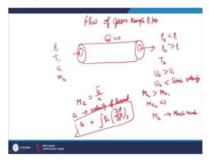
Now, in the next aspect, we will consider the flow of gas through pipe, flow of gases through pipes. Now, here we are having a pipe like this, here the initial conditions are  $P_1$ ,  $T_1$ ,  $U_1$   $Ma_1$  and Q is equal to 0, here the final condition are  $P_2$  is less than  $P_1$ ,  $P_2$  is the greater than  $P_1$ , these two are the conditions  $T_2$ ,  $U_2$  is greater than  $U_1$  or  $U_2$  is less than sonic velocity  $Ma_2$  is greater than  $Ma_1$  and  $Ma_2$  is less than 1.
