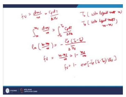
So, we can calculate the fraction of liquid vaporized like
