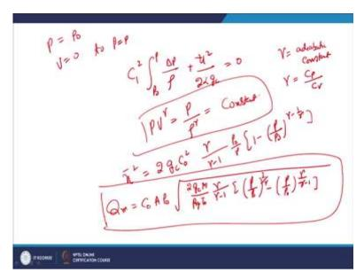
Now, if we combine the both the equation and integration from integrate from P is equal to  $P_0$ , V is equal to P to P is equal to P then we will have
