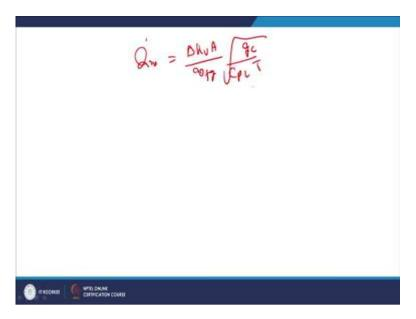
Now, reducing the equation for vapour mass flow rate then
