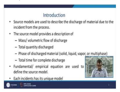
The source model provides a description of mass or a volumetric flow of discharge. The total quantity of discharge, because sometimes you need this information to assess the safety aspect
