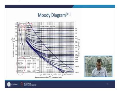
Now, here is the Moody's diagram, which tells you about the, this is a depiction of a relative roughness factor epsilon by d with respect to the Reynolds number that is Re u upon d with the friction factor F. So, you can have a different you can calculate or you can find out based on your material in question then you can find out the friction factor either with the help of a
