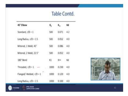
And here in this particular table the 45 degree elbow is enlisted with respect to the  $K_1$ ,  $K_{\infty}$  and  $K_d$ . The standard, long radius, etcetera, threaded, flanged and different descriptions likewise.
