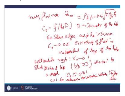
The mass flow rate Q<sub>m</sub> is equal to
