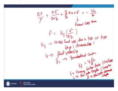
So, for incompressible fluid the mechanical energy equation can be written as
