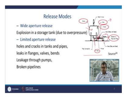
Now, while considering the basic source model, there are seven things which we need to know that is the flow of liquid through a hole because if you consider the previous one, what is the flow of a liquid through hole? And consider this scenario is bit different from the scenario at this point. Then flow of liquid through a hole in tank, flow of liquid through pipes, flow of vapour through holes, flow of gases through pipes, flashing liquid and a liquid pool evaporation or boiling.
