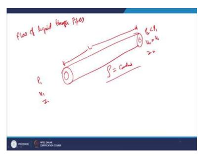
Now, let us consider another thing that is the flow of liquid through pipes. Now, here is a pipe like this which is having the length L, rho, let us take that rho is constant, through pipes, my initial conditions are  $P_1$ ,  $u_1$ ,  $Z_1$  and the final conditions are  $P_2$  is which is less than  $P_1$   $u_2$  is equal to  $u_1$  and  $Z_2$ , here we have taken this thing that " $\rho$ " is constant. Now, let us take say that pipe transporting liquid is shown in the figure.
