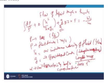
Now, let us consider first thing that is the flow of liquid through a hole. So, basically this particular thing is attributed to the mechanical energy balance equation which describes the various energy forms associated with the flowing fluids. So, this is the basic mechanical engineering equation, mechanical energy balance equation
