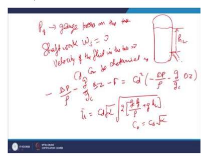
So, the assumptions we what we have taken, that is Pg is the gauge pressure on the tank. I am again redrawing the tank figure over here, here is the hole, hole, this is the liquid level this is hL. Now, external gauge pressure is equal to atmospheric pressure, the shaft work  $W_s$  is equal to 0 and the velocity of the fluid in the tank, of the fluid in the tank is equal to 0, so discharge coefficient  $C_d$  can be determined as
