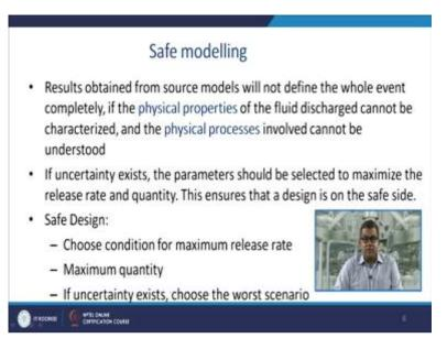
So, while we consider the safe modelling, the result obtained from source model will not define the whole event completely. Now, if the physical properties of the fluid discharge cannot be characterized and the physical process involved cannot be understood. So, if any kind of uncertainty exists, the parameter should be selected to maximize the release rate and quantity.
