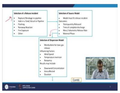
Now, let us have a look of these incidents, there are variety of incidents listed in this block that is a selection of release incident. Sometimes rupture or breakage in pipeline, sometimes a hole in a tank or a vessel or a pipeline, flashing may create a problem means from high pressure zone to the low pressure zone it may create a problem, sometimes runaway reaction may cause a problem, sometimes maybe the fire exposure creates a problem and others which may be enlisted in several aspects.
