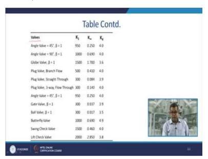
Now, in this slide we have the different valves like angle valve, globe valve, plug valve, gate valve, ball valve, butterfly by valve, swing valve, lift check valve and the values of K1,  $K_{\infty}$  and  $K_d$ . So, in this module we have discussed different aspects of source model and specially applicable for the liquid and liquid system. So, we have discussed the flow of liquid through a small hole, cracks, etcetera.
