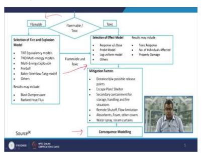
Then while, we considering the flammable or a toxic substances we can enlist two different type of scenario. So, let us have a look of the flammable aspect then the selection for the fire and explosion model you may have a look of the TNT equivalency, Trinitrotoluene equivalency model, TNO multi energy models, multi energy explosion there may be a chances of fireball then Baker-Strehlow the tang model, then different other models.
