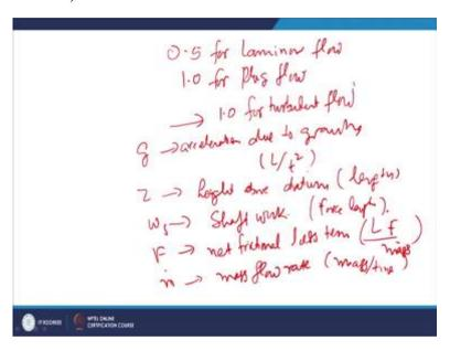
Usually alpha is having the value of 0.5 for a laminar flow 0.5 for laminar flow and 1.0 for plug flow it tends for to 1.0 for turbulent flow. Now, g is the acceleration due to gravity having the units in terms of length times square, z is the height above datum and length unit, Ws is the shaft work that is the force length, F is the net frictional loss term that is length force upon the mass and m is the mass flow rate that is mass per unit time.
