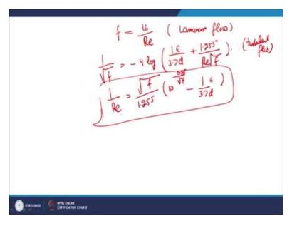
So, for a laminar flow, the fanning friction factor is given by
