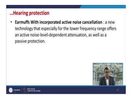
Some earmuffs with incorporated active noise cancellation, these are new technology that are especially for the lower frequency range; offers an active noise level dependent attenuation as well as passive protection.
