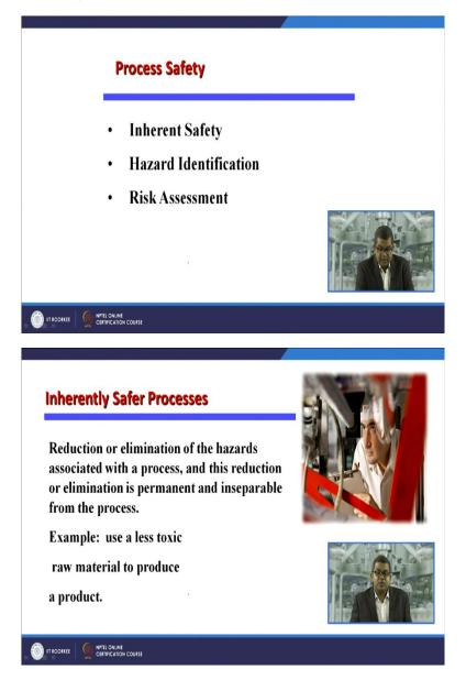
Now as far as process safety is concern, there are three integral part, inherent safety, hazards identification, risk assessment, now inherent safety that is reduction or elimination of hazard associated with the process and this reduction or elimination is permanent, inseparable from the process, first and foremost example is use a less toxic raw material to produce a product,
