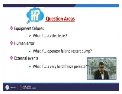
Sometimes equipment failure, what if, if a valve leaks? Human error, what if, if operator fails to restart pump? External events, what if, if very hard freeze persists or storm may occur? So you need to carry out the what if analysis, these are the simple question areas, you may be high localized in terms of question, what if the raw material contains impurities, sometimes the
