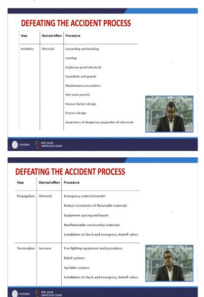
Now there are various tools to defeat the accident process initiation, these are the various procedures in listed over here like you need to diminish all those thing, then grounding, bonding, inerting, explosion proof electrical, appliances, etc, propagation, it should be diminish, it should be decrease, you must have an emergency like emergency material transfer, reduce inventories and so on, that you can devise on your own based on technical knowledge and technical competency.
