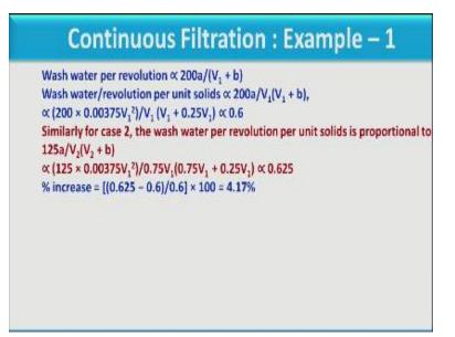
So wash water rate per revolution is proportional to 200 x rate of washing that is a/ $V_1$  + b, so wash water required per revolution. Similarly wash water per revolution per unit solid is proportional to 200 x a /  $V_{1}(V_1$  + b), now here you can see we have defined per unit solid but we are considering volume over here because volume will be associated with the solid which is forming the cake. Therefore we can use this per unit volume, instead of per unit kg of solid.
