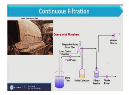
So if you see this particular slide here rotary drum vacuum filter is shown which we have just described, now if you see this figure here we have the knife which continuously removes the sludge or removes the cake which is formed over the drum which is shown over here, and after
