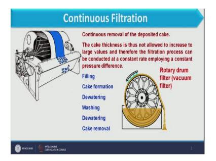
So in continuous filtration we go for continuous removal of the deposited cake the cake thickness is thus not allow to increase to large values and therefore the filtration process can be conducted at constant rate employing a constant pressure difference, now if you remember the batch process where we have define two phenomena first is the constant rate and second is the constant pressure, now pressure why we increase the pressure because after some time when the filtration is carried out.
