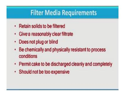
Now here we have the filter media requirements, so what of quality we should see as far as the filter media is concerned and these are the filter media should retain solids to be filtered. So filter media has to retain the solids that is the  $1^{st}$  requirement,  $2^{nd}$  give a reasonable clear filtrate, it should block the solid particle to pass or retain the solid particle and filtrate very clear filter we should get.
