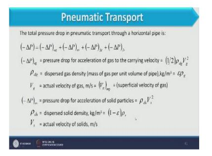
Now here we have total pressure drop in pneumatic transport through horizontal pipe these are different pressure drops and details of these pressure drops are showing in this slide and once we calculate value of total pressure drop we can calculate total power consumption utilized in pneumatic transport, now here we will discuss one example on pneumatic transport.
