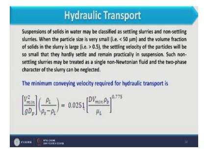
So when the particle sizes very small if it is less than 50 micro meter and volume fraction of the solid in slurry is large that is greater than 0.5 the settling velocity of the particles will be so small that they can hardly settle and remain practically in suspension. So what happens when we have
