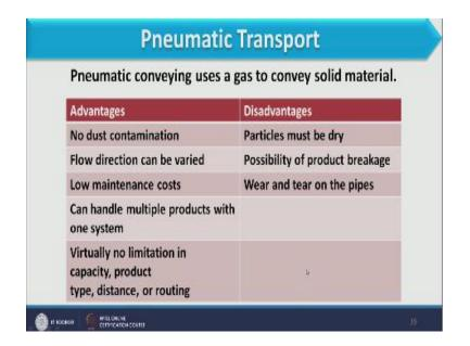
Advantages are no dust contamination flow direction can be varied because we can go for smallest or any route we can go through or we can take any term because that is pneumatically transported low maintenance cost it can handle multiple products with one system because pneumatically it has to transport so it will not a contaminated the inner level of the pipe so we can handle multiple production in the same, we can handle multiple products in the same system or same pipe line.
