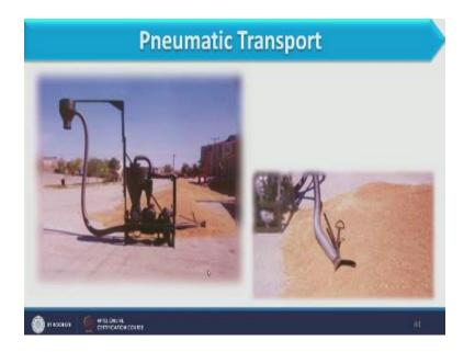
Like if you see this is basically wheat and the we have to pack the wheat that can be pack through pneumatically because from here it takes the wheat and here we put some container where this wheat can be stored, so in this way is storing of wheat or packing of wheat can be done pneumatically, now here we have summary of the lecture now this summary of the lecture. (Refer Slide Time: 23:06)
