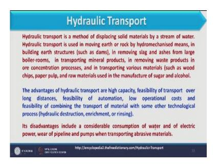
Now let us start with hydraulic transport as we have discussed that in hydraulic transport the mode is water or carrier is water, so when we have to transfer the solid we have to make slurry in the water and then that slurry will be transported through pipe so that is, that happens in hydraulic transportation. Now here we will discuss some of the advantages and disadvantages of hydraulic transportation.
