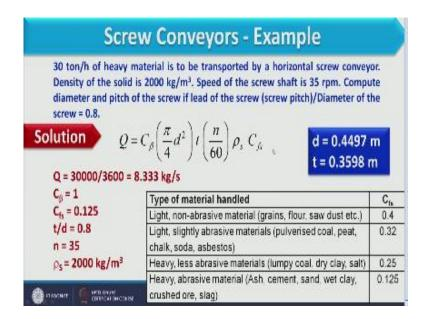
Now here we will discuss one small example where 30 ton per hour of heavy material is to be transported by horizontal screw conveyer density of the solid is 2000kg/m<sup>3</sup> speed of screw shaft is 35 rpm what we have to calculate is the diameter and pitch of this screw if lead of the screw
