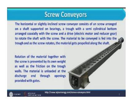
Now in this slide if you see this diagram what is this, this is showing image of a screw conveyer now what happens in a screw conveyer if you see its structure when we consider outer shell of this that is nothing but the semi cylindrical shape. So for a screw conveyer usually we use semi cylindrical bottom or sometimes we also use a square box for transportation for placing this screw.
