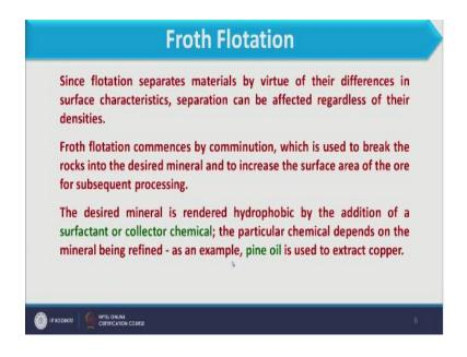
Since floatation separates material by virtue of their differences in surface characteristics, separation can be affected regardless of their densities. So the density of the compound will not affect the separation process only surface characteristics of the compound will matter. So froth floatation commences by comminution, which is used to break the rocks into desired minerals and to increase the surface area of the ore for subsequent processing.
