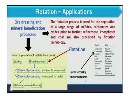
Now as far us flotation application is concerned the main application of this process is in ore dressing and mineral beneficiation process how we go for ore dressing, with this is the flow chart which speaks about recovery of metal from ores, so if we say the ore dressing what is the meaning of ore dressing is, we have to separate the material which are involved in the ore, so what should be the steps of this that is shown through this diagram.
