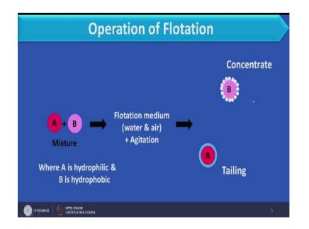
Now as far as operation of floatation is concerned here through this slide I will speak about the operation which is involved in flotation, so if you see this slide here I am having material A and material B so to demonstrate the flotation process I am considering binary mixture and here as far as material is concerned we have taken material A as well as B, These materials should be mixed before starting the operation.
