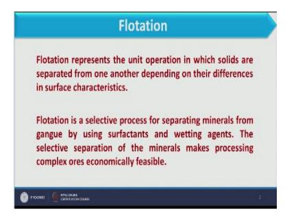
Therefore flotation represents the unit operation in which solids are separated from one another depending on their differences in surface characteristics so you see here because we want to separate the component from the bulk of component or from the bunch or from the bulk so some characteristics we need to separate on which bases it should separate so here the surface characteristics of a component of a material will be used to separate the material from the mixture.
