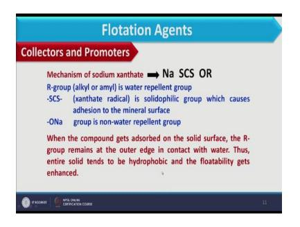
So here we will see the mechanism of sodium xanthate so that you can understand what happens. Here we have sodium xanthate that is Na SCS OR. So if you consider this compound here the Rgroup which is available over here that works as a water repellent group and this is alkyl or amyl group, it works as water repellent. Xanthate radical that is SCS is solidophilic group which causes adhesion to the mineral surface. And ONa group is non water repellent.
