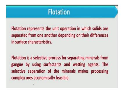
So the selective separation of the mineral makes processing complex or economically feasible, so whatever we are considering that is the complex ore or complex mixture and this selective process give economic solution to that because we can get the separation one by one after heading few surfactants or few agents and that will not be that much costly, so therefore it is economically viable also.
