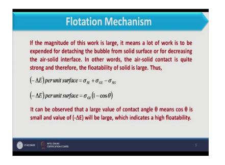
So if the contact angle is small liquid will advance over the surface of the solid, since the surface force is holding the bubble and liquid together will be weak, so when contact angle will be lesser, so after some agitation, after some vigorous agitation bubble can be separated from the solid and liquid will enter between solid and bubble, so it will reduce the wettability. So if we want compound to be floated, so if you want compound to be floated the contact angle should be large.
