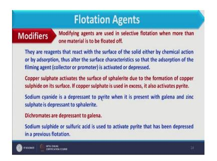
Now what is the purpose of modifier? These are used in selective floatation when more than one material is to be floated off. So here you see when we are having the mixture of compound and we have to separate these compound one by one, so we have to decide the sequence in which they should be floated off. So among the whole material only one we should float off, other we should not.
