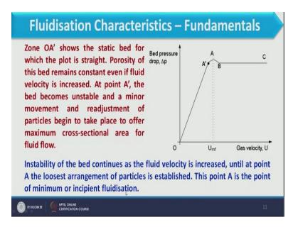
So instability of the bed continues as the fluid velocity is increased until at point A the loosest arrangement of particles is established. So you see at point A the particle may start losing its arrangement and at point A the bed becomes fluidized or this is the condition where minimum fluidization this condition we can called as minimum fluidization condition.
