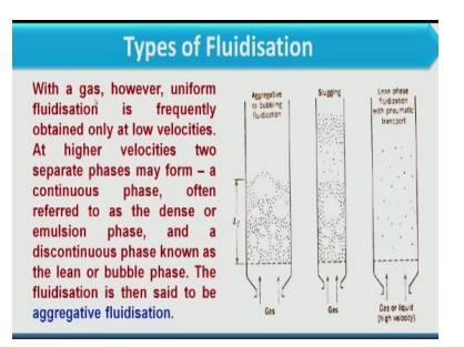
Further if you see this figure in the first figure we have movement of gas so what happens over here when we this happens after minimum fluidization condition achieved after that when we increase the velocity of gas what happens the bubbles are formed inside the bed so particle will not be uniformly distributed but these are placed some more the bunch of particle is placed and some one position.
