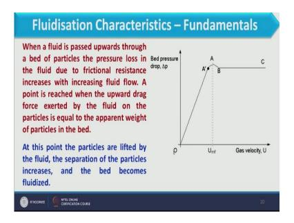
So for proper distribution is for proper distribution of fluid we provide distributor plate at the bottom over which bed space so distributor is important necessary in fluidized bed. Now here we will discuss the fluidization characteristics that is fundamental of fluidization if you consider this curve here we have bed pressure drop verses gas velocity.
