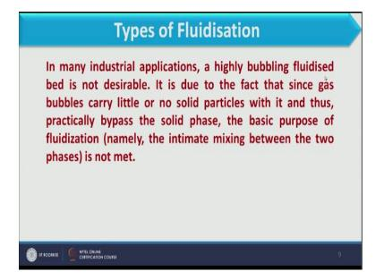
Now in many industrial applications a highly bubbling fluidized bed is not desirable. It is due to the fact that since gas bubbles carry little or no solid particles with it and thus practically bypass the solid phase, the basic purpose of fluidization is not met. So what happens we usually do not consider or do not desire for bubbling fluidization or aggregative fluidization because in that case the gas which has passed through the bed.
