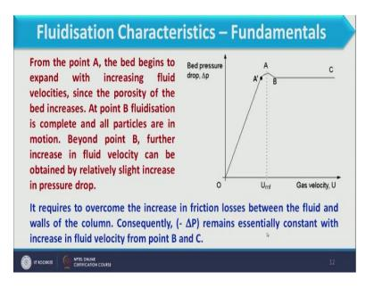
And then we can calculate what is the minimum fluidization velocity that experimentally so the force balance across the fluidized bed dictates that the fluid pressure los across the bed of particles is equal to the apparent weight of the particles per unit area of the bed. So total balance when we want to do should be like this pressure drop equal to weight of the particles – buoyancy force on particles and that should be divide by bed cross sectional area.
