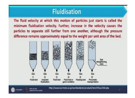
The fluid velocity at which this motion particles just starts is called minimum fluidisation velocity that we have already discussed in the last slide further increasing velocity causes the particles to separate still further from one another, so once we have we will achieve the minimum fluidisation condition where particle will coming into the fluidized state and further increase velocity will separate particle from each other.
