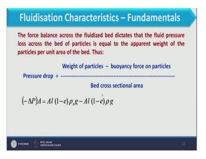
So when we are putting values over here you see pressure drop is  $(-\Delta p)A=A(1-e)p$  g-Al(1-E)p g what is Al is total volume of the A is cross sectional re and l is the height of the bed so thi is the volume of the bed 1-e is fluid section so Al-e is the total volume of the solid in the bed and e can multiplied by this row it will give the mass of the solid into g.
