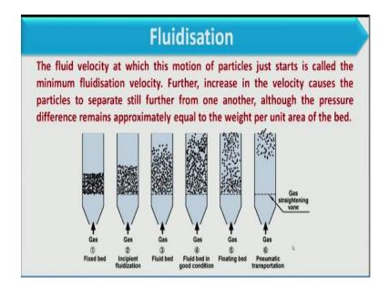
So here we have different conditions of fluidization if you want to study more you can go through this web link now we will discuss different types of fluidization what are the different types of fluidization, mainly it is categorized in two way first is the particulate fluidization and second is the aggregative fluidization, so what happens.
