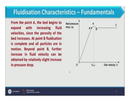
So it requires to overcome the increase in friction losses of the column consequently pressure drop remains essentially constant with increase in fluid velocity from point B and C so this is the whole pressure for the as well as the fluid velocity and we can observe from this we can draw this graph with the experimental data.
