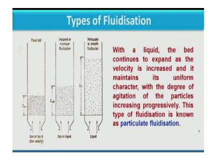
When you see this figure, in figure 1 when gas or liquid flows through the bed and when velocity is less so when velocity is less it will not start moving particle will be at static position itself, so the total height of the bed that should be denoted by Lm, that is the initial height of the bed now further increase in gas velocity when all when drag forces will be equal to the apparent force of the bed it will start expanding and when it will reach to the minimum fluidization condition.
