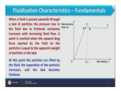
So when this condition is achieved particles it will be start may be in the position in the bed and bed will start expanding at this point the particles are lifted by the fluid, the separation of the particle occurs and further increase in the velocity the separation of the particles increases and the bed becomes fluidized.
