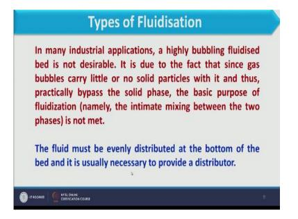
But cannot be achieve the bubbling fluidization and that's why bubbling fluidization is undesirable in the industry cases. So the fluid must be evenly distributed at the bottom of the bed and it is usually necessary to provide a distributor. So what happens for uniform, movement of through the bed the fluid should passed through the bed not from one portion itself. (Refer Slide Time: 27:01)
