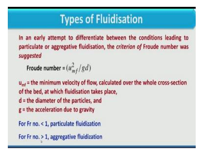
In an earlier attempt to differentiate between condition leading to particulate or aggregative fluidization so here you see we have discussed two type of fluidization the particulate fluidization and aggregative fluidization now what happens that what was the condition through which we can define that this is the particulate fluidization and this is the aggregative fluidization to define this condition we have one dimension less number and that we call as Froude number.
