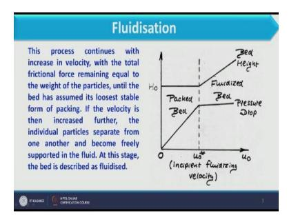
Further this process continues with the increase in velocity with the total frictional force remaining equal to weight of the particle until the bed as assumed it is loosets stable form of packing. So what happen further increase in velocity further allows particle to leave it is a stable state and go further moving state and when we further increase the velocity the individual particle separate from one another and becomes freely supported in the fluid.
