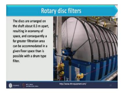
In this image you can see the disc and how this disc are attached through the shaft that you can see in this figure, now each section this is one section each section is associated with this pipe if you see here this is connected with this pipe so whatever filtrate is collected because cake is formed on this surface on both side of the disc And filtrate which is collected is pass through this shaft.
