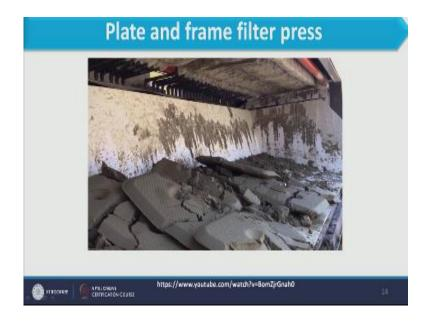
And this is the type of the cake which is the deposited on the each filter cloth is available on the both side of the frame so here we have the cake formation on the both side of the flame occurs and her in this slide we will discuss in that one digits and in the plane filter.
