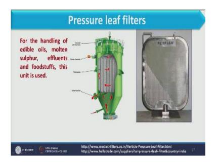
And the pipe if you see all these leafs are concert with this pipe where the filter which is filtrate the falling in between the inside the leaf it s collected through this pipe.
