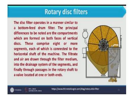
Next equipment we have is the rotary disc filter it is also operated under vacuum but as we have seen in rotary drum filter the cloth is available at outer edge of the drum, however in disc filter what happens cloth is covered to the disc and that disc is associated one and that disc is attached to the shaft very near to each other. So if you see this image we can illustrate how it is working if you see this disc it has different sections and each sections sucks water.
