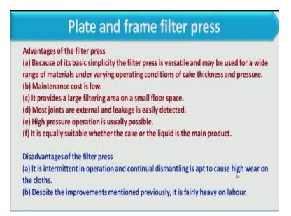
So because this filtration on the batch in the cycle in the dismantle thus the arrangement of the cloth and the frame will be carried out in the life will not be very large in the mention because in the dismantling clewing is required in this stress, now next filter we have in the pressure leaf filter if we see we have the image of this what happens in the leaf on that different leaves if you see in the one figure.
