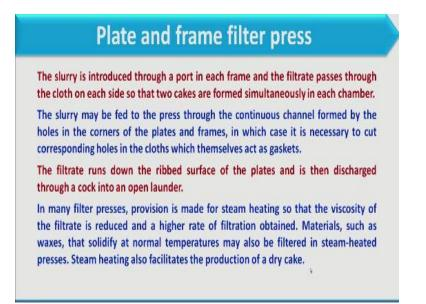
So if you see this slide here in this above three point it shows the basic principle which I have already explained to you. And further we should note that in many filter presses provision is made for steam heating, so that the viscosity of the filtrate is reduced and a higher rate of filtration obtained. Materials such as waxes that solidify at normal temperature may also be filtered in steam heated press.
