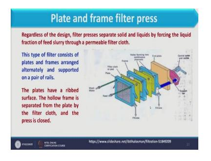
So regardless of the design filter press is separate solid and liquids by forcing the liquid fraction of the feed slurry through a permeable filter cloth. So here basically we use the filter cloth as a filter media and it blocks the solid on the filter media and let the filtrate penetrate through the media. So it separate basically solid and liquid for that purpose, for which purpose filtration is known.
