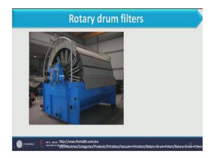
This is how in industry looks like this you can see from this image you can go through in detail to this website and you see this is basivclkly8 the knife which continuously removes the cake.
