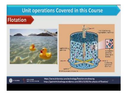
The idea what is flotation that when material floats over the surface that will call has floatation? Now this second figure speaks about the particular operation as far the chemical engineering is concern. So we will concede the flotation. (Refer Slide Time: 32:16)
