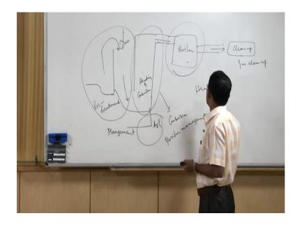
So, in this flow sheet one system is required for the combustor that is there and we need to feed the material inside it we need to feed the material inside it and that is done by some means that is done by some means. So, the solid material which is coming with some cranes or some management it is lifted and put in the incinerator put in the incinerator and homogenization of the solid waste is required.
