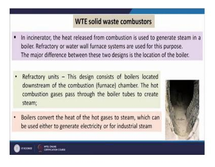
In another case, the boiler is used from this form is that is refractory unit the gas is going out and it enters to the boiler and then in boiler the steam is generated. So, after this in this module we will start discussion in the next module on different types of incinerators gas clean of etcetera.
