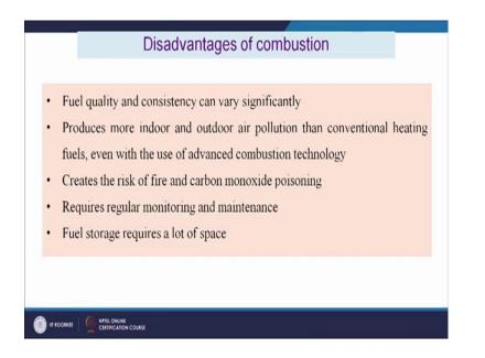
But it has some disadvantages also like say fuel quality and consistency can vary significantly produces more indoor and outdoor air pollution than conventional heating fuels and even with the use of advanced combustion technology creates the risk of fire
