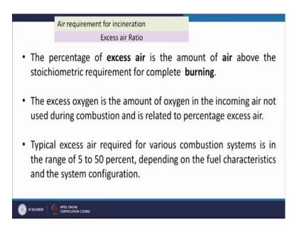
Next excess here how can we calculate excess here; obviously, the amount of oxygen which is supplied into the incinerator with respect to this stoichiometric requirement that will not be used that will not be used.
