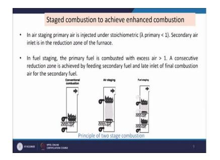
So, in this case how it is different the air staging primary air is injected under stoichiometric. So, this is under stoichiometric la lambda is less this is 1 less than; 1 less than, but here lambda is high. So, it is greater than 1; 1 to 1.5 in between 7. So, this is greater than 1.
