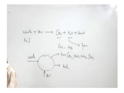
So, if we take waste and air or oxygen it will give us CO2; water and heat now this CO2, H2O will be in gas form, if waste contains nitrogen sulphur waste, we will get here SO2 we will get NOX.
