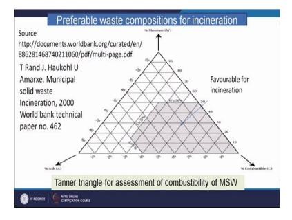
Now, how can you select the solid waste for this incineration purpose? We can do it depending upon 3 properties one is ash content, another is moisture content and another is fixed carbon or carbon content. So, here this portion is basically suitable for incineration and this is tanner triangle, this is used for the assessment of combustibility of (Refer Time: 26:17) solidest. Now let us see the flow sheet how the solid waste is converted to energy through the incineration route.
