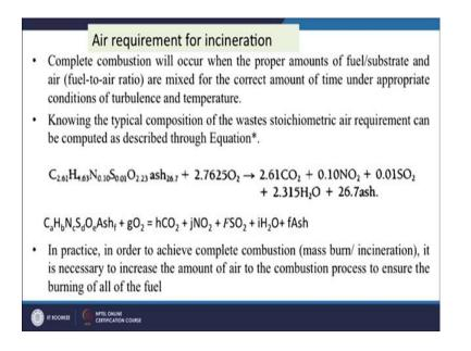
And this is generalized say CaHbNcSdOe and S, this is the molecular formula of the waste or the material that has to be combusted with say this is f and g HO2. So, then it will give us h CO2, NO2 plus SO 2 plus f ash and these will be h this equal to say j and f plus I H2O.
