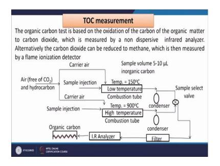
So, that way when we will be using only 150 degree centigrade temperature then we will get inorganic TOC and when we will be using nine hundred centigrade we will be getting both by difference we will get the organic TOC. So, these are the very important parameters for waste water on energy point of view that is DO BOD cod and TOC.
