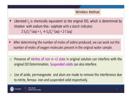
So, when the iodine concentration is reduced and it is converted to iodine at end point that color will change it will be colorless. So, we will get the end point and then from the end point calculation we will get the strength and volume of thiosulfate used and correspondingly iodine reacted with this thiosulfate we can calculate by this reaction and equivalent amount of oxygen is also present in the waste water. So, this is the method for the determination of DO through Wrinkler's method.
