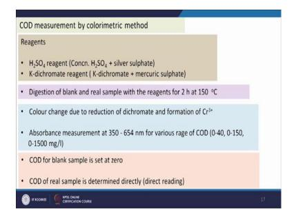
So, if we use a light of certain absorbance which is applicable for Cr 3 plus then the absorbance value will give us the indication of the oxygen used or the organic compound present and there is some calculations and some softwares are available in the machines that convert these absorbents to cod and directly gives us cod value for blank test this is put 0 and for real sample this is determined directly.
