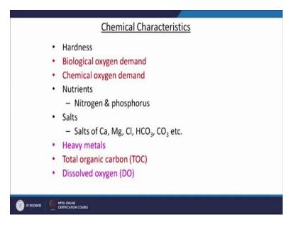
Along different chemical characteristics we will see the hardness biological oxygen demand; BOD, chemical oxygen demand; COD, nutrients, nitrogen and phosphorus present in waste water different salts and different ions, Cations and anions, heavy metals total organic carbon and dissolved oxygen.
