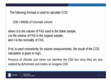
So, nitride interference can be eliminated by using sulphamic acid and to reduce the chloride interference mercurus sulfate is used.
