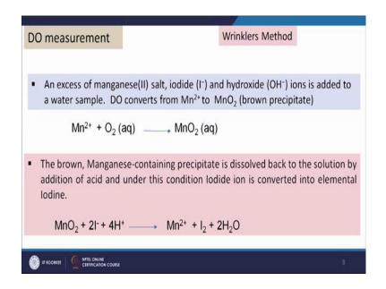
So, when this acid is added to dissolve the MnO 2 in the solution then that Mn, MnO 2 reacts with iodide ions in presence of h plus and forms iodine now here one mole of iodine is produced from one mole of MnO 2 and one mole of MnO 2 is produced from one mole of oxygen. So, amount of iodine which is produced now in the solution is equivalent to the amount of oxygen in terms of moles present in the waste water or any water sample.
