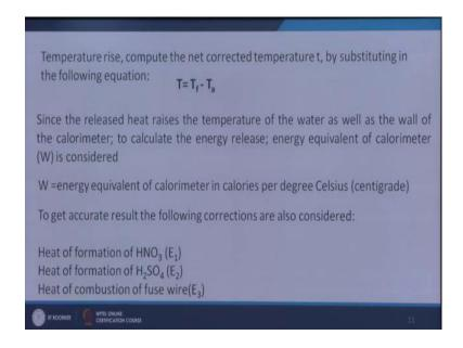
So, how can be measure this is equal to M c p d t mass C p into del T, del T can be measured that is T f minus T a, final temperature minan initial temperature we can measure the T equal to that is del T t equal to T f minus T a; and then what is our C p, M C p say we have M 1 of the bomb M of the bomb into C p of the bomb M C p into del t plus M of the water in the bucket C p of the water in the bucket into del T; that is equal
