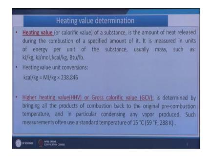
If we combust some amount of waste it will generate some amount of heat. So, that heat can be used for different applications.
