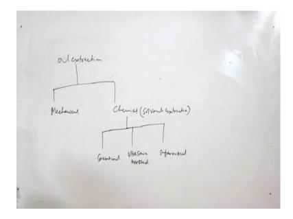
So, we can write say oil extraction, it is having mechanical and it is chemical, that is solvent extraction that may be of conventional or may be of ultrasonic assisted or may be supercritical. So, that way also we can represent this method. Now will see these are 2 pictures the oil press and this is solvent extraction. Normally for the solvent extraction soxhlet apparatus is used. So, as show in the figure this is a soxhlet apparatus the working of this apparatus is like this.
