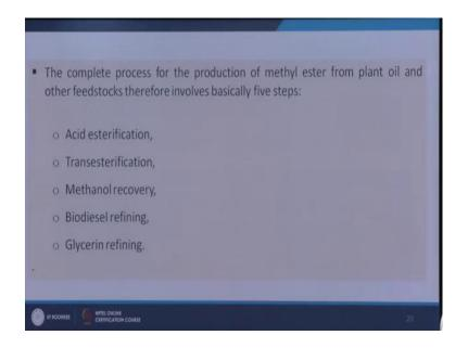
And we have basically these are the steps, acid esterification transesterification methanol recovery biodiesel refining and glycerin refining. So, up to this in this part and the next part will discuss in next class.
