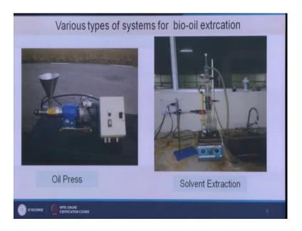
Say as we see here, here is the solvent. We heat it the vapor the vaporized solvent will go up come here is condensed. So, liquid will form. So, liquid solvent will drop here solids will be kept here and finally, liquid will come here the liquid mixing between the liquid and solids and solid liquid will be going to this beaker through syphon action. So, this not very clear I am drawing here.
