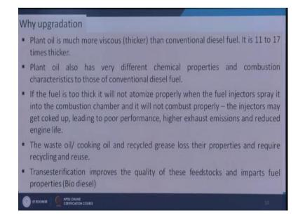
So, these are the major difficulty with the bio-oil. So, bio-oil which is produced from oil seeds or some other waste oil seeds. So, those cannot be directly used, that has to be converted or upgraded through the transesterification that is what the importance of transesterification there is for bio-oil which is produced from the waste oil seeds.
