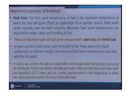
So, there will be some momentary flash. So, that is called flash point. So, if we raise the temperature then fire will catch. So, that will be the fire point. So, fire point and flashpoint are the important properties of the fuels. So, there are 2 methods for the measurement of flash point one is closed cup and another is open cup method.
