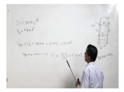
So, V g s t plus V D we are getting V g s t plus V D we are getting how much 305 into 40,that is equal to 12200 liter or 12.2 meter cube we can get 12.2 meter cube, and another way of discussed again that V g s t plus that is equal to 0.8 into v. So, what will be V g s t plus V D is equal to 0.8 into v.
