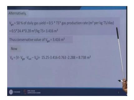
Now, alternatively we also know that V g s t can be calculated on other thumbs rule that is 50 percent of daily gas yield that is 0.5 into TS or total solid into gas production rate that is meter cube per kg TS per day. So, these value is equal to 0.28 as given in the statement. So, 0.25 TS is equal to 24.4 as per the statement given we have calculated and then this is equal to 3.416 meter cube. So, V g s t one formula is giving us 3.416 meter cube.
