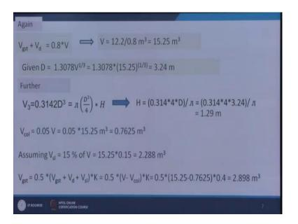
So, H is equal to 1.29 meter. So, by this calculation we are getting H is equal to 1.29 meter. Now we have got the value of H, now we need to calculate the V collection, what is the V collection that is 5 percent of V, what is sludge collection sludge volume that is equal to 15 percent of V.
