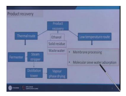
So, this is these are on the thermal route. So, for the recovery of the ethanol from the solid residue as well as the waste water in the fermenter we have 2 types of operations or 2 types of routes one is thermal route another is membrane based route.
