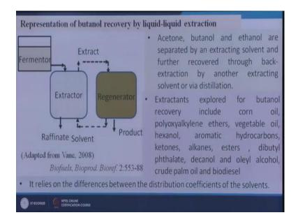
Next, liquid-liquid extractions; so fermenter broth can be contacted with some liquid which will be having some specific butanol capturing capacity. And this works on this the difference between the distribution coefficients.
