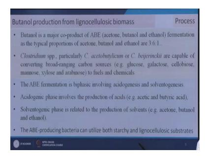
Now, we are coming on butanol production. So, butanol can be produced through the fermentation, but here the process will be slight different. The separations of the butanol from the media will also be slightly different from that of ethanol production.
