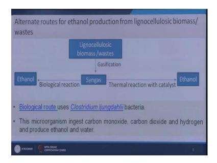
Now, we will discuss some other routes which are applicable for the production of ethanol. So, here two routes have been shown one is by the gasification the waste material can be converted to syngas. And that syngas can further we converted to ethanol through catalytic reaction we have discussed in previous modules that once syngas is produced that can be converted to ethanol or methanol or any other higher alcohol.
