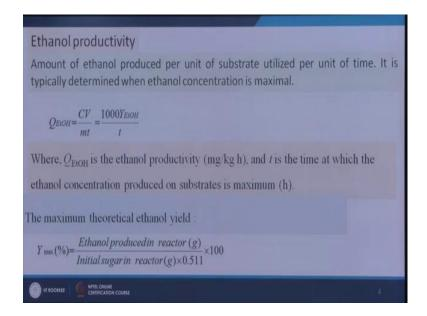
Now, what is the ethanol productivity? If we can determine the ethanol yield, then if we divide it by time then we will get the ethanol productivity. The definition of ethanol productivity is the amount of ethanol produced per unit of substrate utilized per unit of time.
