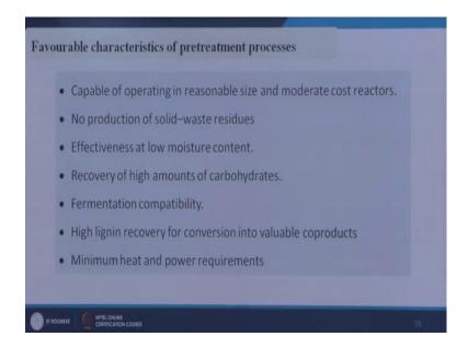
Then capable of operating in reasonable size and moderate cost reactors no production of solid waste residues, we do need any solidate residues in this step and effectiveness at low moisture content and recovery of high amounts of carbohydrates. So, we have to recover high amounts of carbohydrates through this process, and fermentation compatibility then minimum heat and power requirements. So, these are some characteristics of this process.
