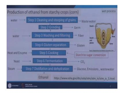
Now, we will concentrate on the production of ethanol from to starchy crops. So, one example is your corns. So, in this case the corn, it contains germ, it contains gluten it contains starch and it concerns bran. So, these are the composition of the corn.
