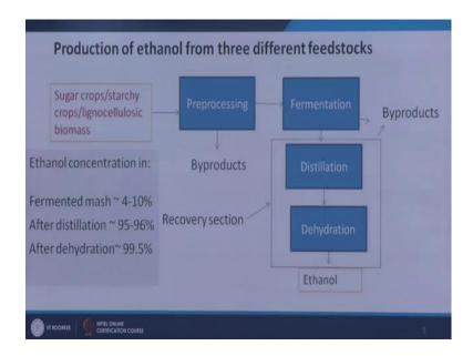
Then production of ethanol from 3 different feed stocks 3 types of different feed stocks basically.
