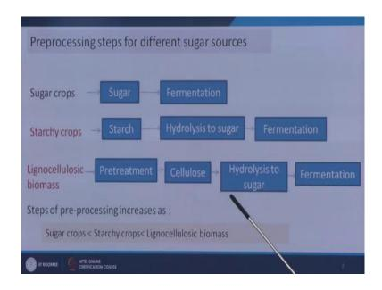
So, this thing already we have discussed. So, if it is a sugar crops, then sugar crops to sugar then sugar to fermentation; simplest method. Then it is starchy crops we will get starch from the starchy crops then starch has to be hydrolyzed to convert it into sugar.
