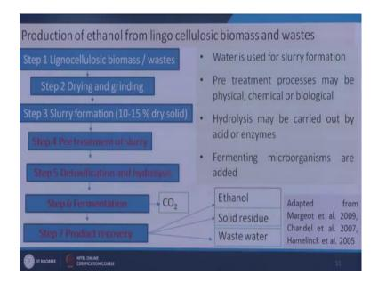
Now, we will see the flow sheets for the production of ethanol from the lingo cellulosic biomass as you have discussed that when the material is lingo cellulosic biomass, it will be requiring stringent preprocessing step that is pretreatment. So, lingo cellulosic biomass and waste after drying and grinding it will go for slurry formation. And then that is 10 to 15 percent dry solids will be there then it will go for pretreatment step.
