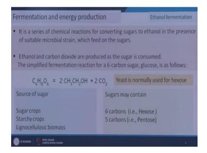
So, what is methanol fermentation? It is a series of biological or chemical reactions for converting sugars to ethanol in presence of suitable microorganisms. And then basically what type of reactions takes place in this case sugar is converted to ethanol and carbon dioxide.
