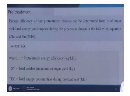
So, if this is the role of the pretreatment step how can we define the performance of this pretreatment step or the energy efficiency of any pretreatment step. So, that is defined as efficiency equal to TSY by TEC, what is TSY is the total soluble sugar yield how much total solve sugar we are getting in kg and total energy consumptions during the free treatment in mega joule, so kg per mega joule that will be the efficiency of this pretreatment process.
