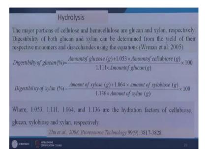
So, this is the part the hydrolysis. The major portions of cellulose and hemi cellulose are converted to sugar. So, what is this cellulose and hemi cellulose? This is having glucan
