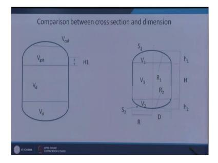
So, here we some example I will show how to correlate these things before that what is the basic difference between the dimension and the cross section if we take the cross section we will get 4 parts gas collection gas storage active digestion sludge.
