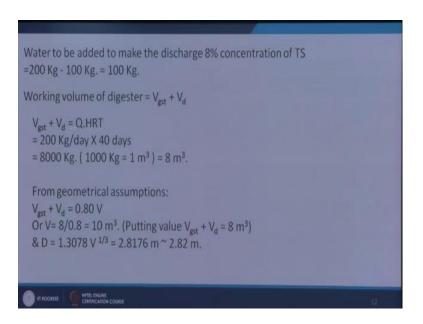
So, working volume of the digester, we will be having working volume is equal to obviously, gas to rate zone plus V d that is active zone. So, V g s t plus V d is equal to Q into HRT.
