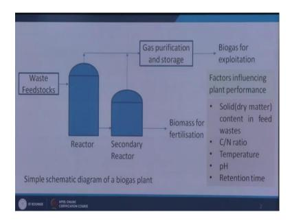
So, now at first we will see the simple schematic diagram of a biogas plant. So, here waste feed stocks its entry into first reactor then second reactor secondary reactor then biomass for fertilizations and biogas for storage and the factors which influence the plant performance are solid content in the feed stock and then C by N ratio temperature pH
