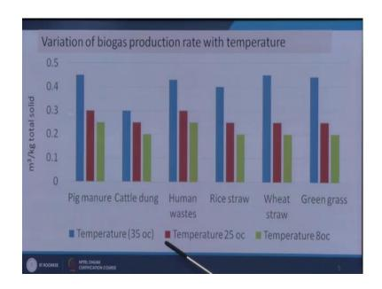
So, we see here in all the cases 35 degree is giving us the higher rate of gas production. So, we will be considering the mesospheric zone there is 35 38 degree centigrade and after considering specific conditions we will find out the sizing of the reactor.
