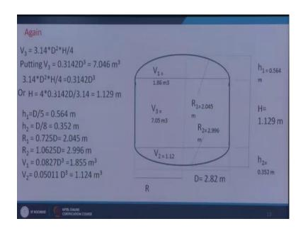
So, next we are having say V 1 V 2 V 3, what is the V 3? This V 3 equal to pi R square H. So, pi into D square by 4 pi into D square by 4. So, this equal 2 and then D equal to how much? We have got D is equal to 2.82 meter. So, if we put the value of D, here D cube when this VV3 is coming 7.046 meter cube and again VV3; we have got from this
