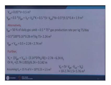
Now, we will say b collection is equal to maximum say 5 percent we are assuming of V. So, 0.05 V equal to 0.5 meter cube and V g s t is equal to 0.5 into V g s t plus V D plus V s l into k that is equal to 0.5 into what is this V g s t? V D and V s l this is equal to total V minus V c o l. So, that is equal to V minus V c o l into k or 0.5 into 10 minus 0.5. So, 9.5; we are getting 0.5 into 9.5 into 0.4; 1.9 meter cube.
