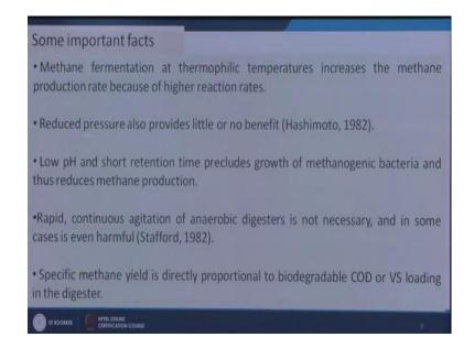
And low pH and short retention time precludes growth of methanogenic bacteria. So, if the pH inside the anaerobic digestion reactor is very less. So, less pH that will inhibit the growth of the mechanogenic microorganisms methanogenic microorganisms reacts well at the pH of seen 0.2 or 7.4 to 7.9 whereas, acidogenic bacteria reacts with would very result gives very good result at 5.4 to 5.9 pH.
