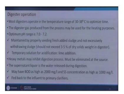
So, these are some conditions which are considered as a optimum conditions like say temperature 30 to 38 degree centigrade pressure seen to 7.2, this is obviously for a single chamber anaerobic digestion only single chamber we will be using a single chamber. So,
