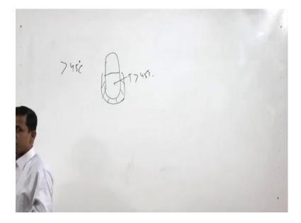
If we want to get the higher rate at say temperature above 45 degree centigrade we have to heat the material inside the digester also above t greater than 45 degree centigrade. So, external heating is required. So, in that case external heating is required.
