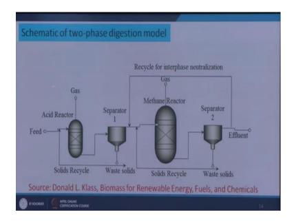
So, this is the schematic of 2 phase digestion model how actually the plant looks likes. So, if you put feed here the acid reactor acidogenic phase gas out it is going to the separation for the sludge and then it is coming supernatant here then the second phase that is methanogenic phase methane production will take place. So, again the sludge will be settled and recycled back in both the cases the sludge can be recycled back or the sludge can be taken out.
