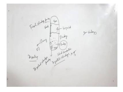
Let us see we have one anaerobic digestion unit we are putting here feed. So, this is a sludge this is a liquid and this is a gas. So, material which is coming inside that is reacted by the microorganisms. So, microorganisms are acting on these substrates which are coming inside it as a result the sludge is formed.
