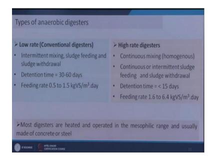
Here that is 15 to 125 feet here we will see types of anaerobic digesters. So, anaerobic digesters can be used as low rate process or as high rate digesters. So, low rate higest digesters means its feeding rate is lower; obviously, 0.5 to 1.5 K g volatile solid per meter cube per day and its detention period is also higher that is 30 to 60 days.
