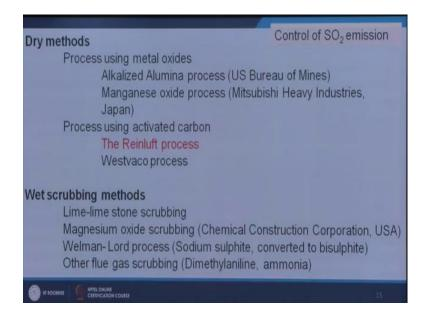
So, this 3 adsorbance has been used by different companies as mentioned here. So, these are available technology dry methods or adoption base methods for the removal up SOx from the gas stream.
