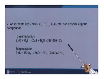
So, all those things we have discussed in the previous module. Now we will be focusing on some control of specific gaseous pollutants like control of SOx emission control of NOx emission and control of CO2 emission. So, control of SOx emissions how the SOx are HO2 emission can be controlled or SO2 can be removed from the gas stream.
