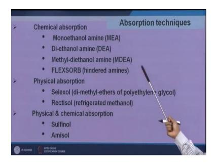
So, those methods are MEA that is monoethanol amine, di-ethanol amine, methyldiethanol amine MDEA and FLEXSORB and then physical absorption Selexol and Rectisol and Sulfinol and Amisol. So, these are the absorption base methods which we have already discussed those are used for the removal of particular gas components. (Refer Slide Time: 24:28)
