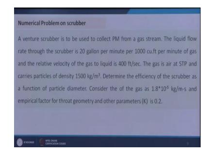
The gas is air at STP and carries particles of density 1,500 kg per meter cube determine the efficiency of the scrubber as a function of particle diameter considered the viscosity of the gas as 1.8 into 10 to the minus 5 K g meter second and empirical factor for throat geometry and other parameters is 0.2.
