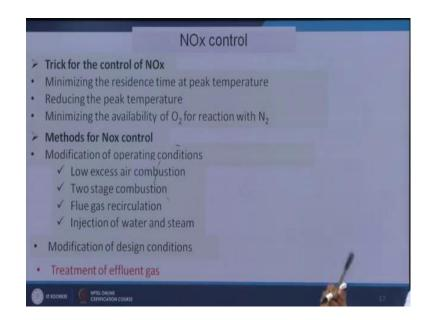
So, we will be giving more emphasis on treatment of effluent gas, but apart from this the NOx emission can also be reduced by the modifications in the methods as well as by applying some tricks there is a higher the temperature more NOx formation takes place. So, if we can reduce the temperature in the reactor.
