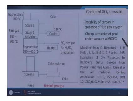
So, this is the flow sheet of the reinluft process is. So, activated carbon is the adsorbent in this case. So, one adsorption column will be there this is adsorption column where we will send activated carbon here it is coke the coke which is made that it cheap semi coke of peat under vacuum at 600 degree centigrade. So, this coke is used at adsorbent and it is put here.
