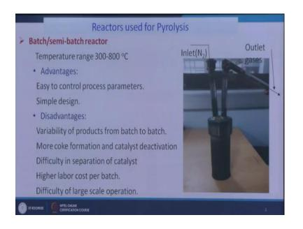
So, first we will discuss on batch type of reactor. So, as soon here this is a batch reactor very lab scale very small scale reactor. So, we here will be putting some material solid plastics if catalyst can also be added then we will heat it. So, pyrolysis will take place and vapor will be going out. So, this route and after condensing here we will be getting the liquid product and nitrogen will be sent to carry the vapors through this.
