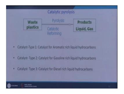
So, this catalyst for aromatic rich hydrocarbon, so here pyrolysis along with catalytic reforming, so they are catalyst are here having some property that can perform the reforming reactions and then products will be liquid and gas phase and the liquid maybe either aromatic rich or gasoline rich or diesel reach depending upon the use of catalyst type if we use one it is aromatic rich if you use catalyst 2 then there is gasoline rich catalyst 3 that will diesel rich.
