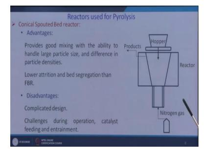
So, next will see another type of reactors which have been reported in literature that is conical spouted with reactor. So, here from the top will put the feed stocks and then from the bottom nitrogen gas and there will be pyrolysis reactions. So, during the pyrolysis reactions will get the vapor.
