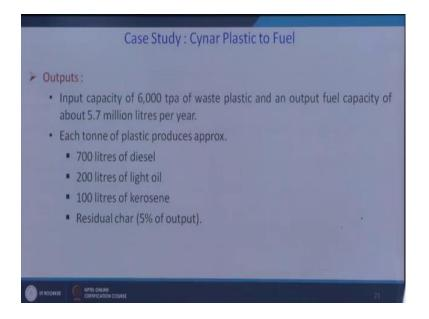
And each ton of plastic produces approximately 700 liters of diesel 200 liters of light oil and 100 liters of kerosene and residual charge is around 5 percent. So, this is one example of the waste to liquid fuel production technology through pyrolysis by Cynar plastics of fuel plastics. So, what is the benefit the benefit is that by this process the emission is reduced significantly.
