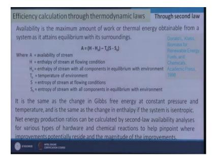
And net energy availability is defined as a is equal to H minus H o minus T into S minus S o. So, H is the enthalpy of stream at flowing condition and H o is a enthalpy of stream with all components in equilibrium with environment. And similarly the S and S o are and T o is a temperature of environment. Now this is similar to del g equal to del H minus t del s. So, it gives pre energy relationship.
