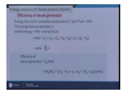
So, we can get HHV that is equal to Q 1 which we have got that is useful energy plus the losses; losses mean some of Q 2, Q 3, Q 4, Q 5, Q 6, Q 7, and Q 8 and Q 9. So, this is the HHV equations.
