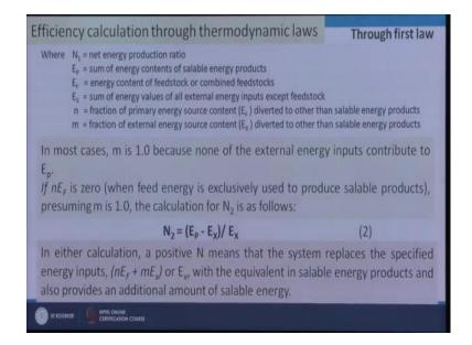
So, this is proposed by this scientist. And normally m is equal to 1 and n is equal to 0, because m is m is what fraction of external energy content diverted to other than salable product. So, this is equal to normally 1 and n is equal to 0. So, N 2 expression is E p minus E x by E x. This indicates that the n p is always positive; that means the energy which is produced that is much more than which is consumed.
