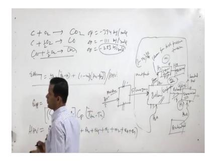
So, that efficiency that is equal to W s by W f into we have got that is H 2 minus H 1 plus 1 minus m 1 into H 4 minus H 3 divided by HHV. So, this is the efficiency of this.
