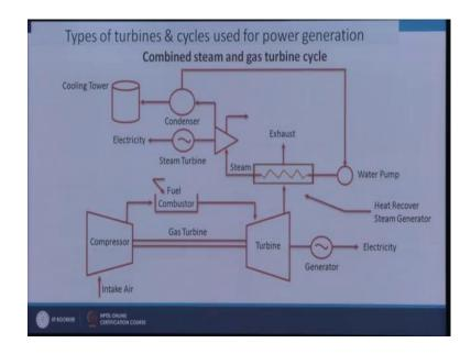
And this is a combine cycles; means steam and gas both turbines is available. So, first the turbine this turbine will work fast gas turbine it will work fast the exhaust of the gas turbine will be used first steam generation and then the condensation will be going on.
