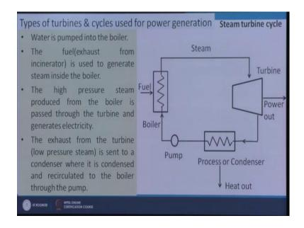
So, here this is the working of this. In case of steam turbine the steam is produced here and it is coming to turbine and then electricity generated. And after condensing this recycle back. Already we have discussed these things.
