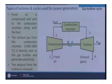
Similarly, the turbine cycles we have also discussed in the first part of this. So, where its sent compressed and then combustion takes place and then the combusted gas is pass through the turbine gas turbine and then we get some work here. And this temperature is around 1500 to 1800 centigrades, we have discussed in the first part of this module.
