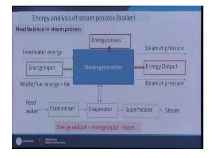
So, our boiler super heater and economizer are three main important parts. So, we have shown here then feed water is coming economizer then evaporator then super. So, this boiler is evaporated, so these are the parts.
