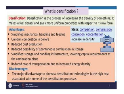
Now, let us see what is the definition of densification? So, densification is the process which increases the density of any material; when it is applicable for fuels that increases the density of the fuel as well as it give some uniform properties like uniform particle size the higher density etcetera.
