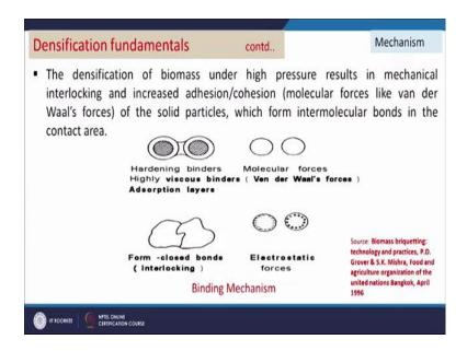
So, for the productions of briquettes we can see we need to put high pressure so that the particles will come closure and will be interlocked, or we can add some binders. So, some materials are there for which binder is essential the some materials are there if we apply high pressure binder is not required, and the binder helps to bind the particles and keep them close.
