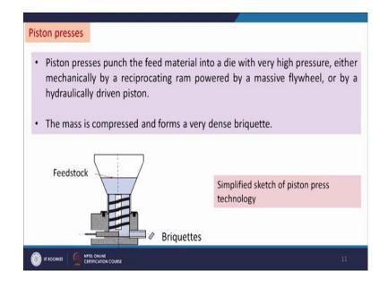
Now, will see how the piston press works? Now see in this slide we are seeing here one piston press. So, material feed is put here the feed is put here in passes through the necks and comes in this position, and this is the piston this piston have forward and backward movement.
