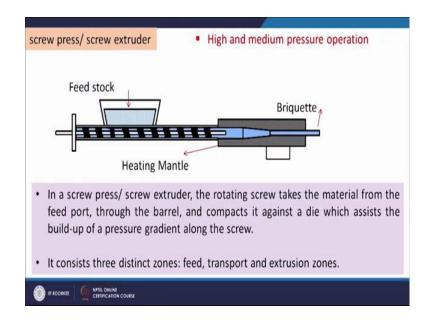
Now, we are coming to screw press or screw extruders; we see here one diagram schematics of the screw extruder. So, feed materials enters into the screw. So, the screw has some shaft which is rotating, this is the shaft it will rotate and due to the rotation the material enters into the screw will get some velocity and it will move forward it will move in forward direction.
