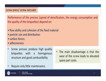
So, this is the mechanism of the production of the briquettes to the screw press; now how the performance of this screw process screw press is dependent, how this performance can be influenced. So, the performance depends upon flow ability and cohesion of the feed materials. The feed materials which is used here what is the flow ability and what is the cohesion properties particle size and distributions.
