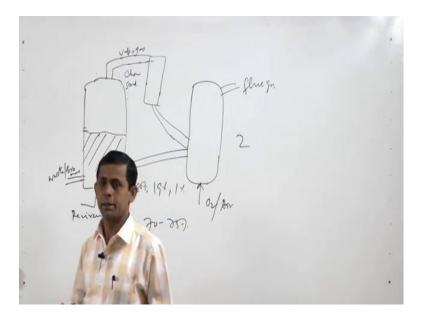
In circulatory fluidized bed reactor, 2 chambers are used. In the first we put biomass or waste and here we put recycling gas re circulating gas re circulating gas where from it comes it comes from the second chamber.
