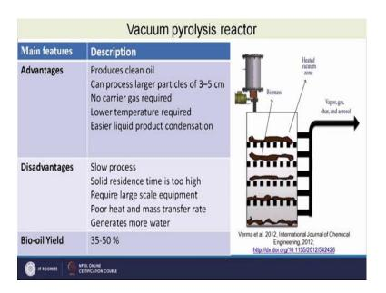
So, this material can be put in different rays and some vacuum is created here. So, that we do not need to provide any inert gas to carry the vapor produced inside the pyrolyzer
