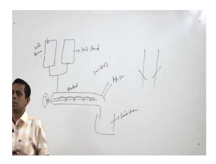
In screw reactor we use to tank, one containing hot sand and another is containing waste or biomass.
