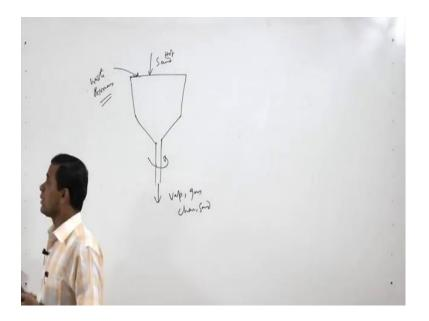
In rotating cone reactor on cones have reactor is used in this cone shape reactor, it is rotated and we add waste or biomass from the top and also sand there is hot sand we also put hot sand and this and there is some scientifically action on it.
