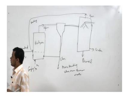
Now, we will see the process flow sheets of the pyrolyzer unit. So, one pyrolyzer we will put biomass and waste that biomass and waste must be pretreated because this will be able to handle certain biomass only. So, that pretreatment is required just like segregations and homogenization etcetera.
