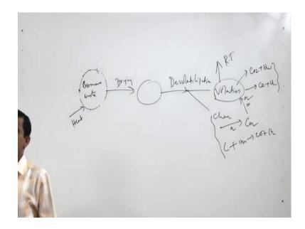
In case of combustion, the volatile first drawing then it is coming to de volatilization that we will give us volatiles and char.
