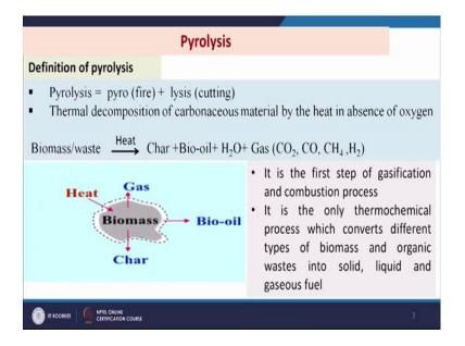
Pyrolysis the word itself gives some idea about it. So, pyro means fire, lysis means cutting. So, this is the process that is thermal decomposition process which decomposes carbonaceous material by the application of heat in absence of oxygen.
