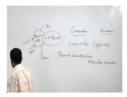
So, if we have some biomass and waste or any carbonaceous feedstock just simply we will apply heat in the combustion and in the gasification, we had to put some other medium that is oxygen for combustion and O 2 and H2O in case of gasification, but in this case we do not (Refer Time: 03:25) to only heat and that heat will give us char that will give us gas and that will give us bio oil.
