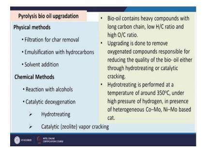
The physical method is filtration for char removal emulsification with hydrocarbons and solved degradation for the chemicals methods reaction with alcohols and catalytic deoxygenation.
