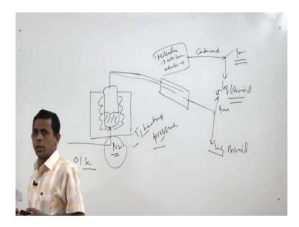
We will get some important information in this figure we have one pyrolysis chamber very small one inside a furnace. So, this furnace will apply heat we will put some material here and where putting here we are heating by coil permitting the material we have put it and then disconnected.
