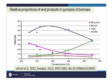
And then bio char decreases with increase in temperature. So, bio chart decreases with increase in temperature and moisture content there is no much change there is no much change in moisture content and gas content increases with increase in temperature gas contents increase with increase in temperature we can explain this phenomena on the basis of the mechanism of pyrolysis we have seen that there are there are primary degradation then further secondary cracking of the of the volatiles.
