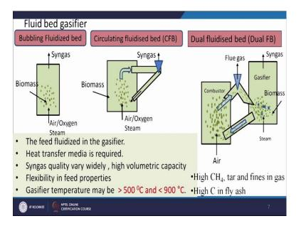
So, this bubbling fluidized bed and circulating fluidized bed the main difference is that the gasifier gasifying agent's velocity is higher in case of circulating fluidized bed and un-converted materials are recycled to the gasifier.
