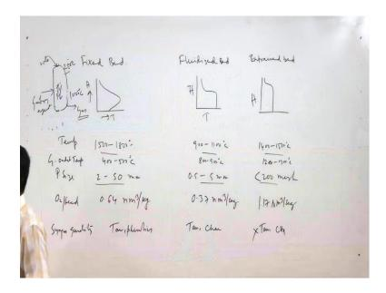
In the previous part, we have seen that for fixed bed gasifier, the temperature is maximum at the combustion zone or coal gasification. And then it decreases this is along height and this is temperature and for fluidized bed. We had seen that the temperature is almost constant and very high, up to certain height of the gasifier, but above that the
