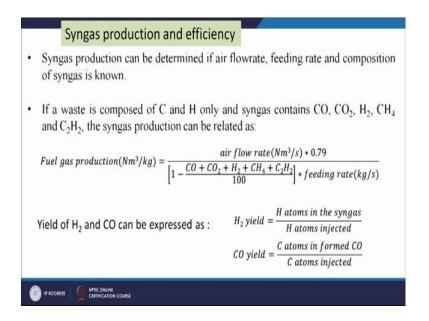
Here some formula is given using which we can calculate the fuel gas production rate if the material the raw material or feedstock contains only hydrogen and carbon and the product gas contains CO, CO 2, H 2, CH 4 and C 2 H 2, then fuel gas or syngas fuel gas or producer gas whatever it may be depending upon the situation.
