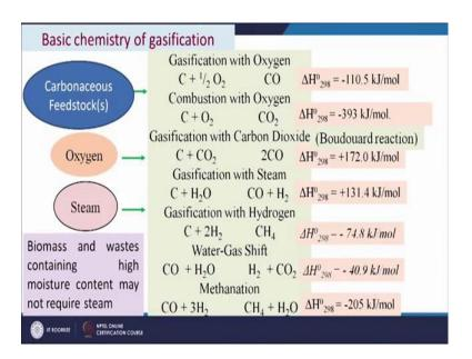
Now, we will see the basic chemistry of gasification. This approach or this chemistry basic chemistry involves the reactions with elemental carbon present in the feedstock with different agents like say oxygen, carbon dioxide, H 2 O and H 2.
